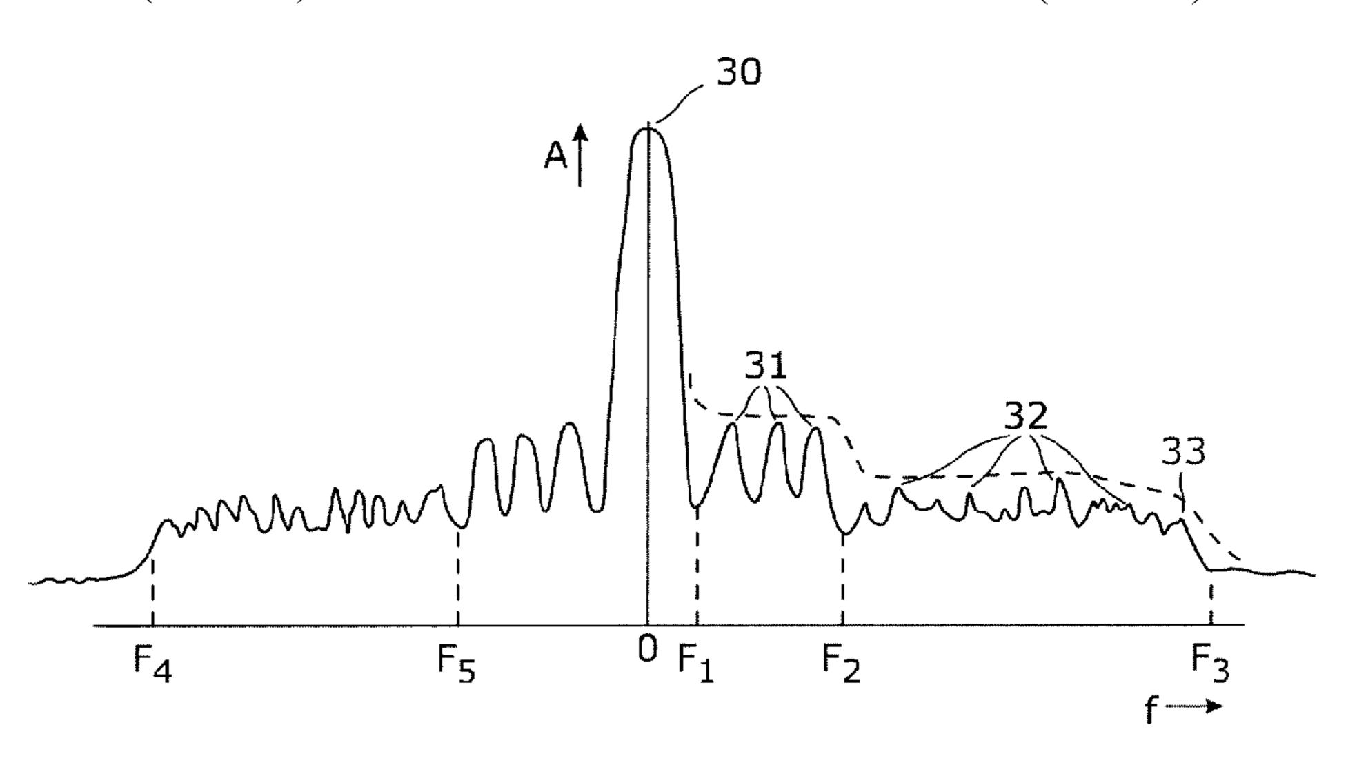
teristic form of the Doppler signals in some instances allow the body return to be implied, thus providing information as to drone velocity.
