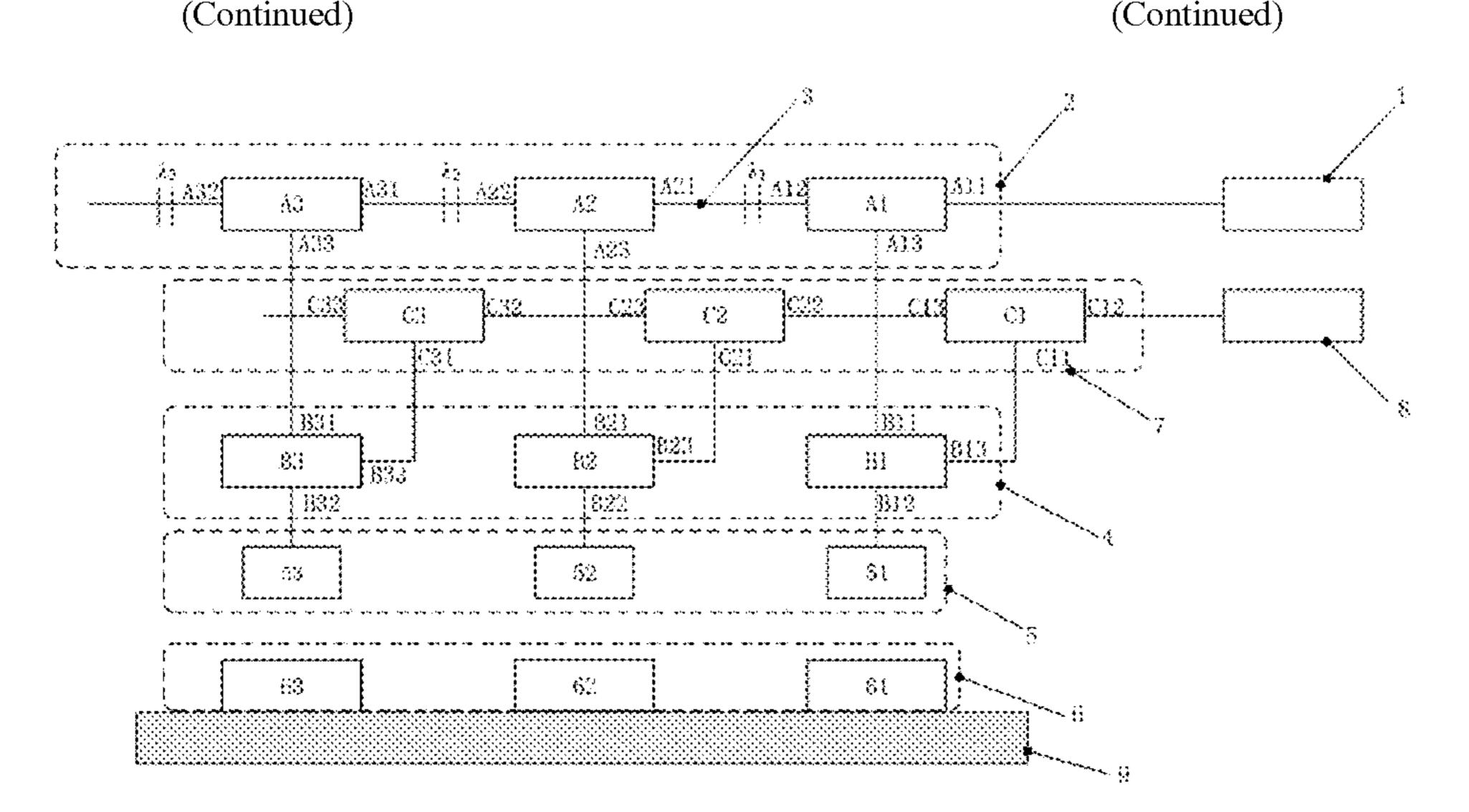
adhered to the working face of the scraper conveyor through first optical fiber circulators, second optical fiber circulators, and collimators. The light with the different wavelengths is then reflected back from the reflecting films, enters the SMF through third optical fiber circulators, and finally enters the optical path analyzer.
