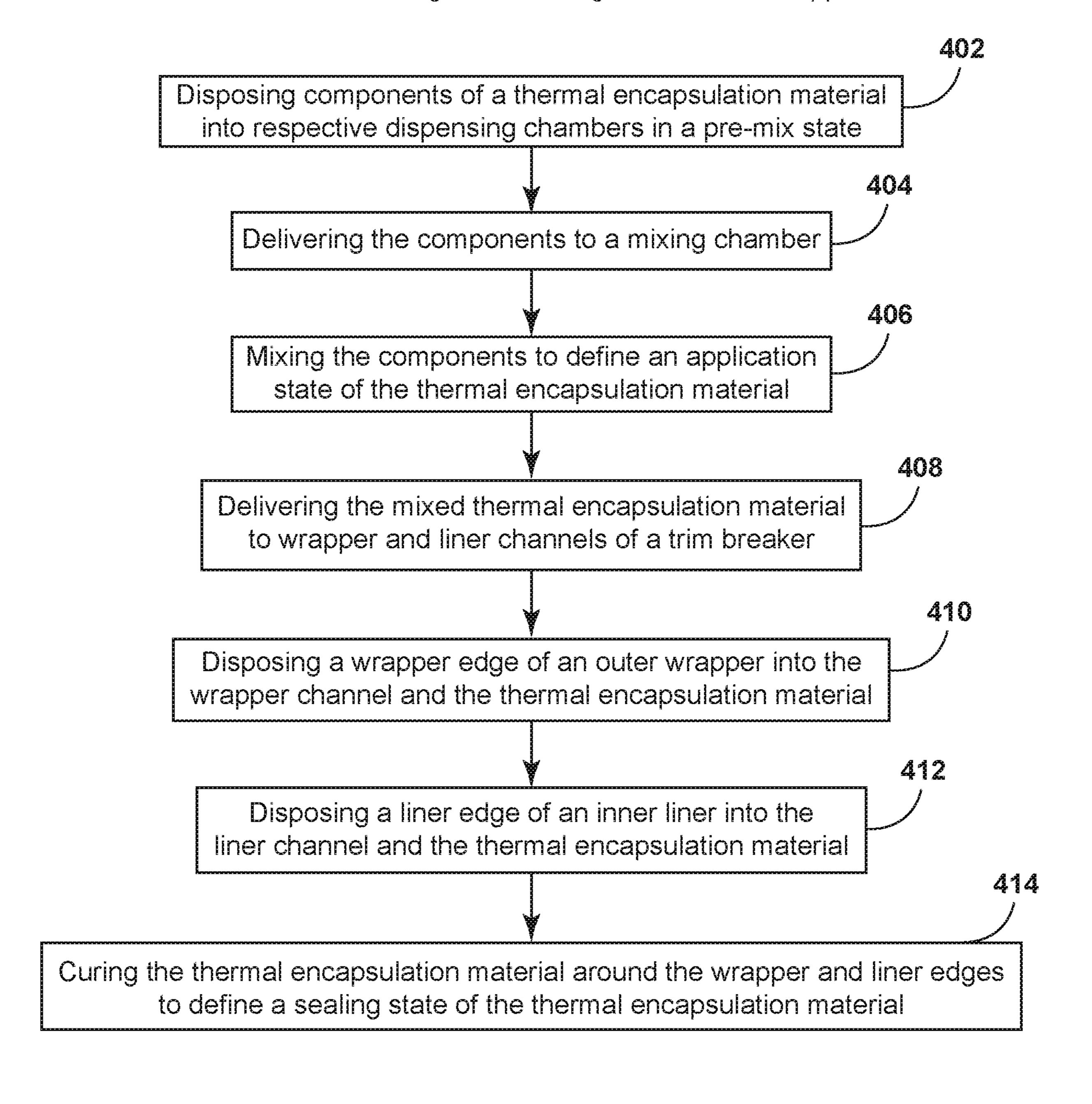
Method 500 for Forming an Insulating Cabinet for an Appliance
