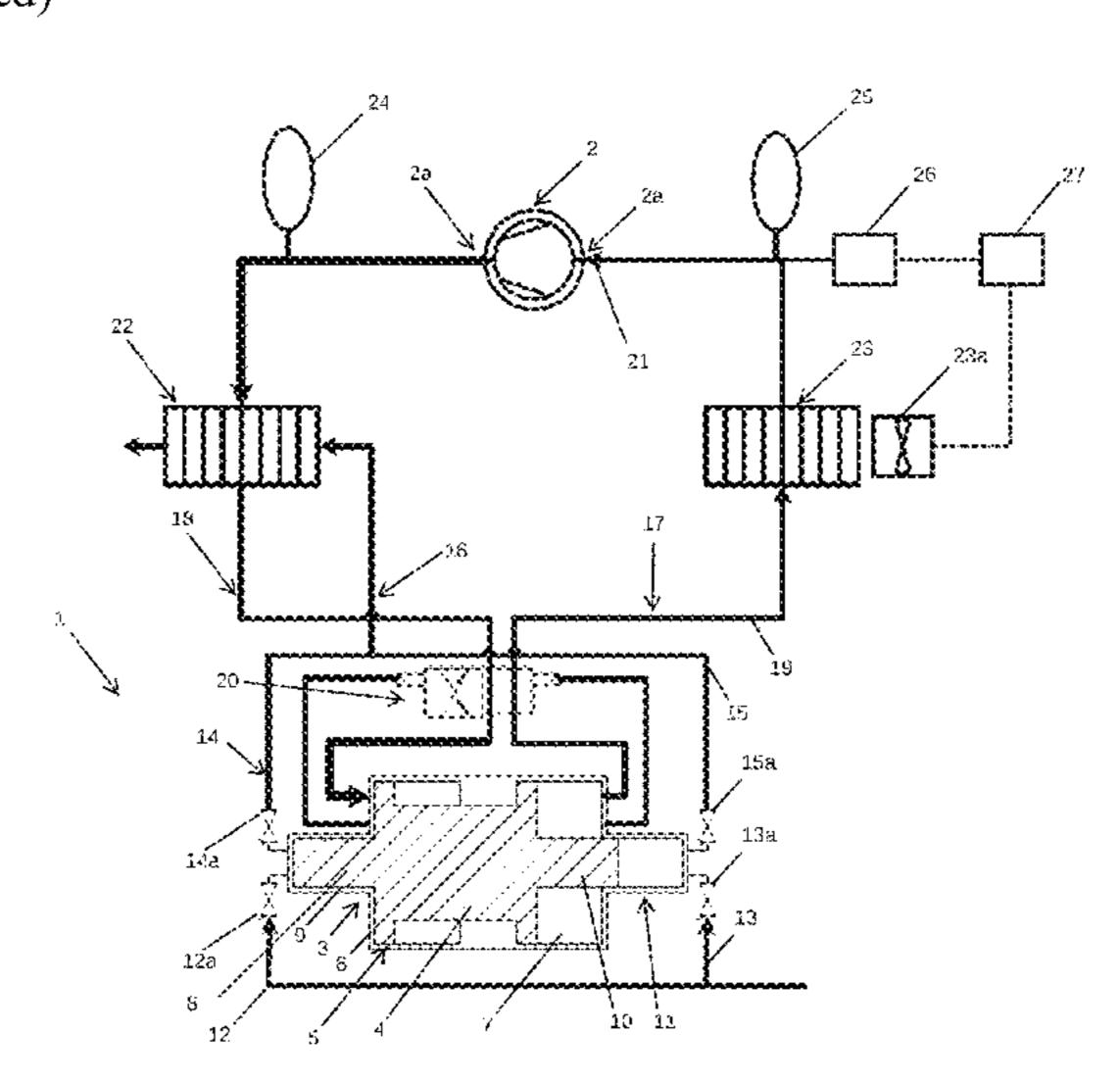
transferring heat from the compressed working medium to the compressed drive medium before the compressed drive medium enters the first cylinder of the drive piston.
