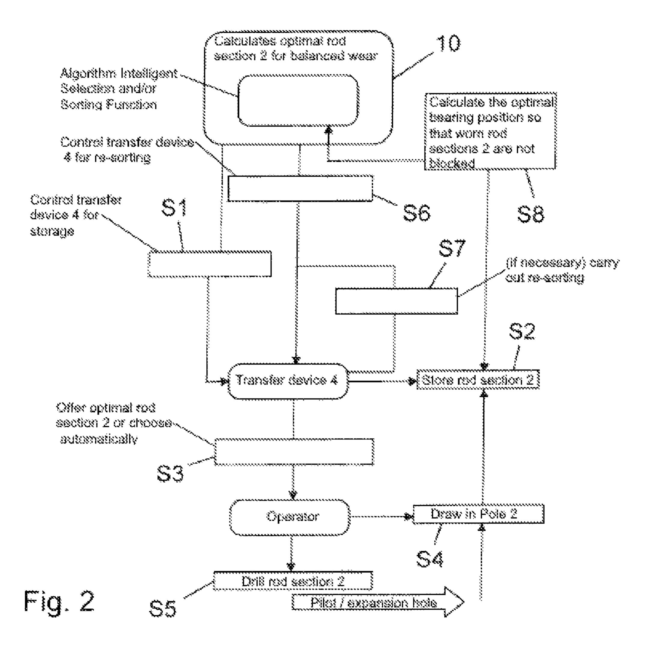
GROUND DRILLING DEVICE, TRANSFER
