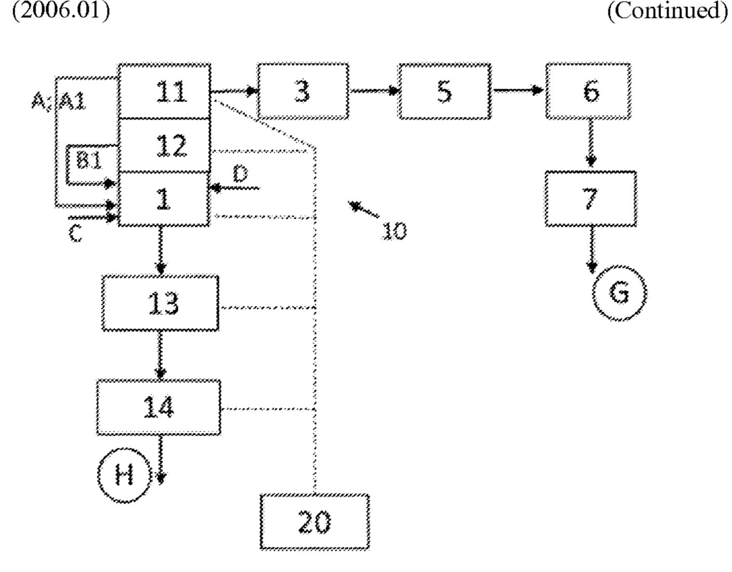
fluidized bed gasification process and upstream of the particle separation unit (11), having a return (B1) for gasification steam (B) that can be coupled to the fluidized bed gasification process. Furthermore, the invention relates to a method for the aftertreatment of at least gases downstream of a fluidized bed gasification process as well as the use of an intermediate cooling unit.
