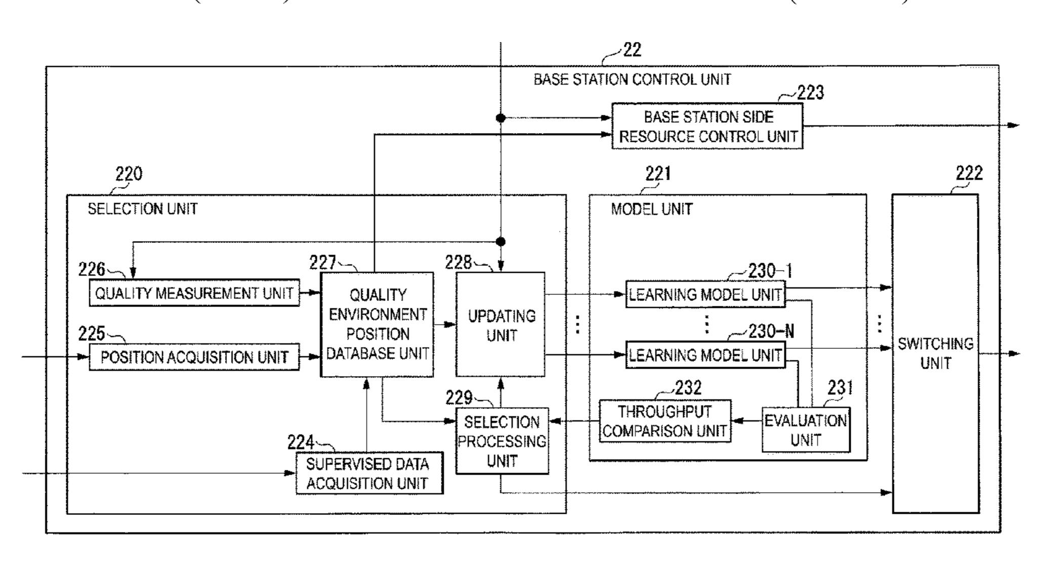
information representing the radio wave environment based on the downlink wireless signal, generating information representing quality of communication based on the learning model data and the information representing the radio wave condition, and controlling the communication resource for the wireless signal based on the information representing quality of communication.
