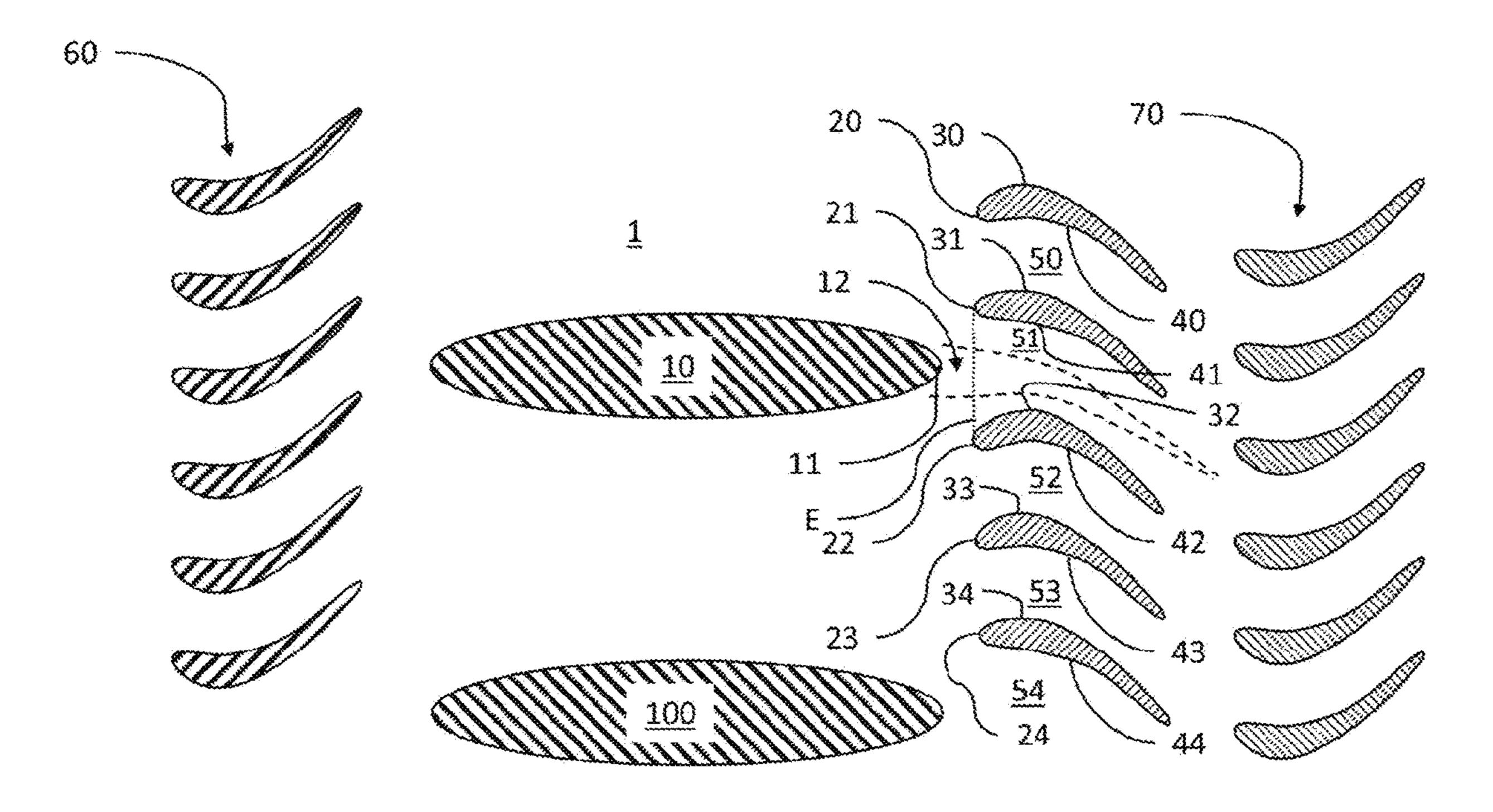
the flow passages is adapted to this support rib, that it is situated downstream of, in order to reduce a pressure loss and/or a vibrational stimulation.
