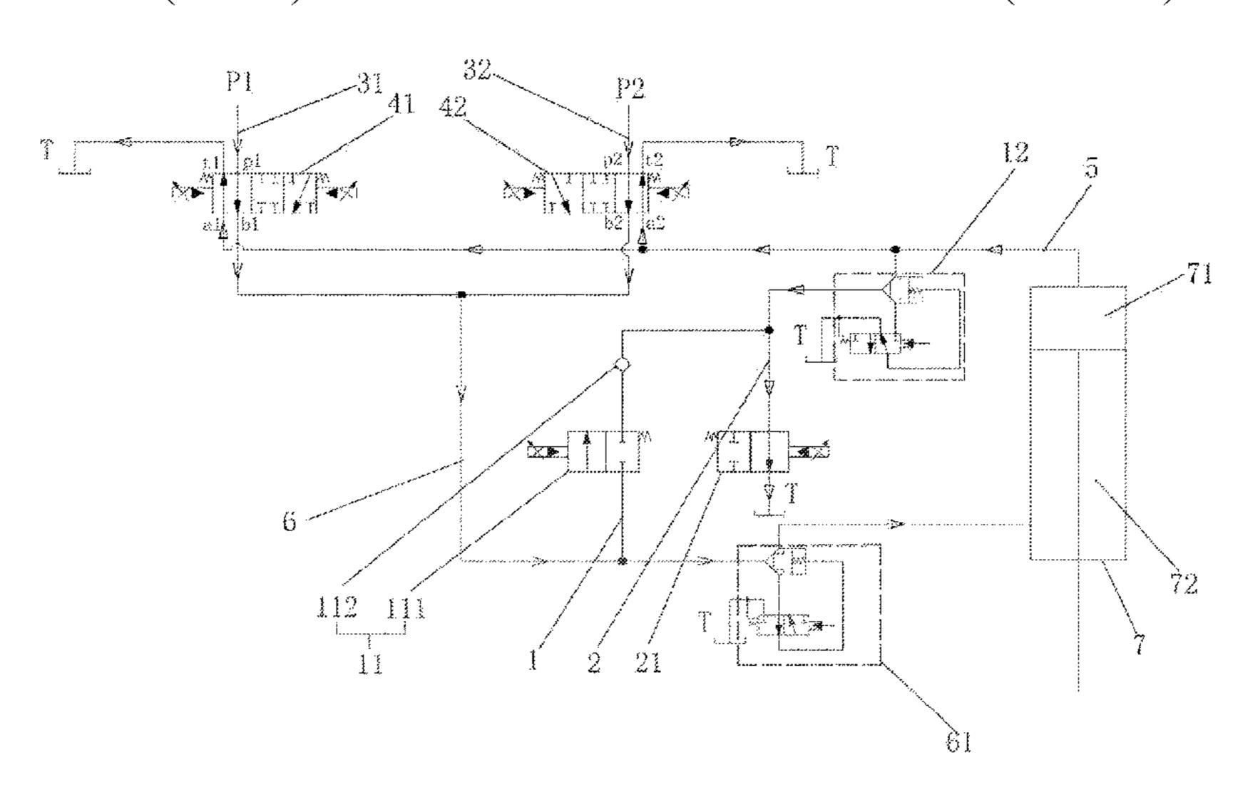
regeneration cut-off oil path when the working device swings outwards. The regeneration cut-off oil path is configured to send the regeneration oil passing through the regeneration valve or the oil discharged from the actuator to other destinations.
