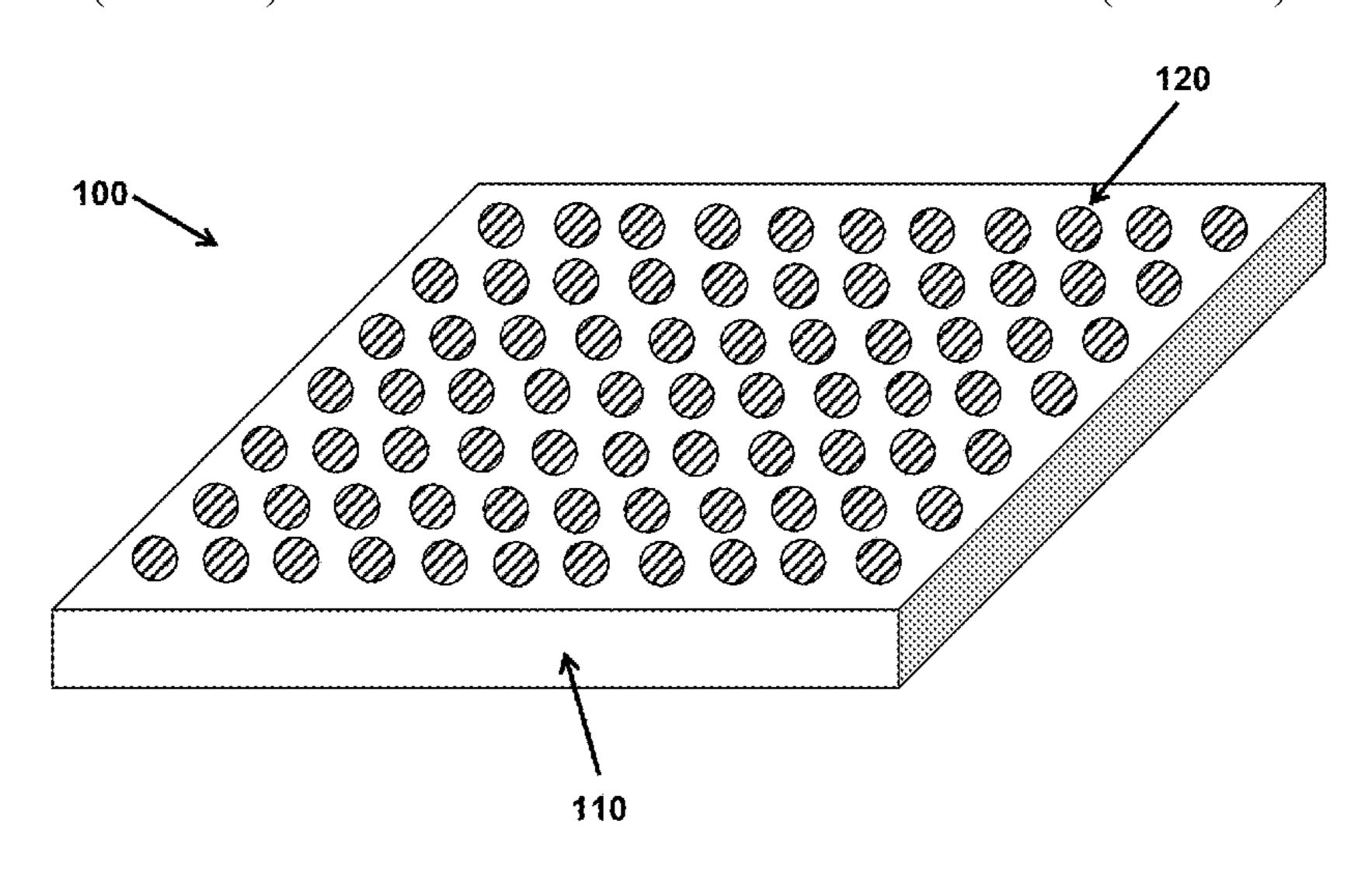
or the second component is a low-surface-energy polymer, and the other is a hygroscopic material. The coatings are characterized by an AMIL Centrifuge Ice Adhesion Reduction Factor up to 100 or more. These coatings are useful for aerospace surfaces and other applications.
