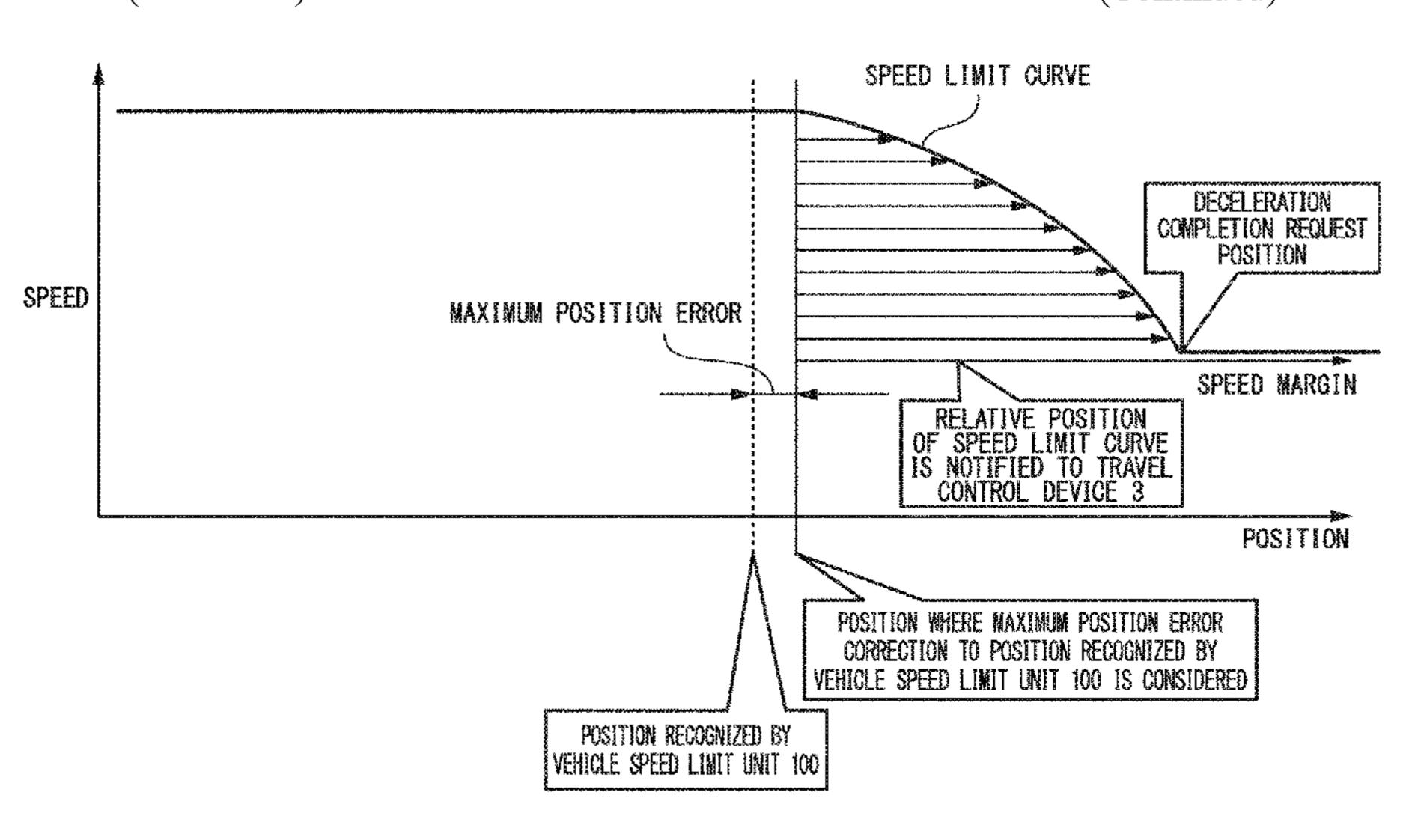
speed limit at each position obtained from the limit information according to the acquired limit information, the current position, and the current speed. The speed command unit is configured to generate a speed command according to the generated travel curve and the current position.
