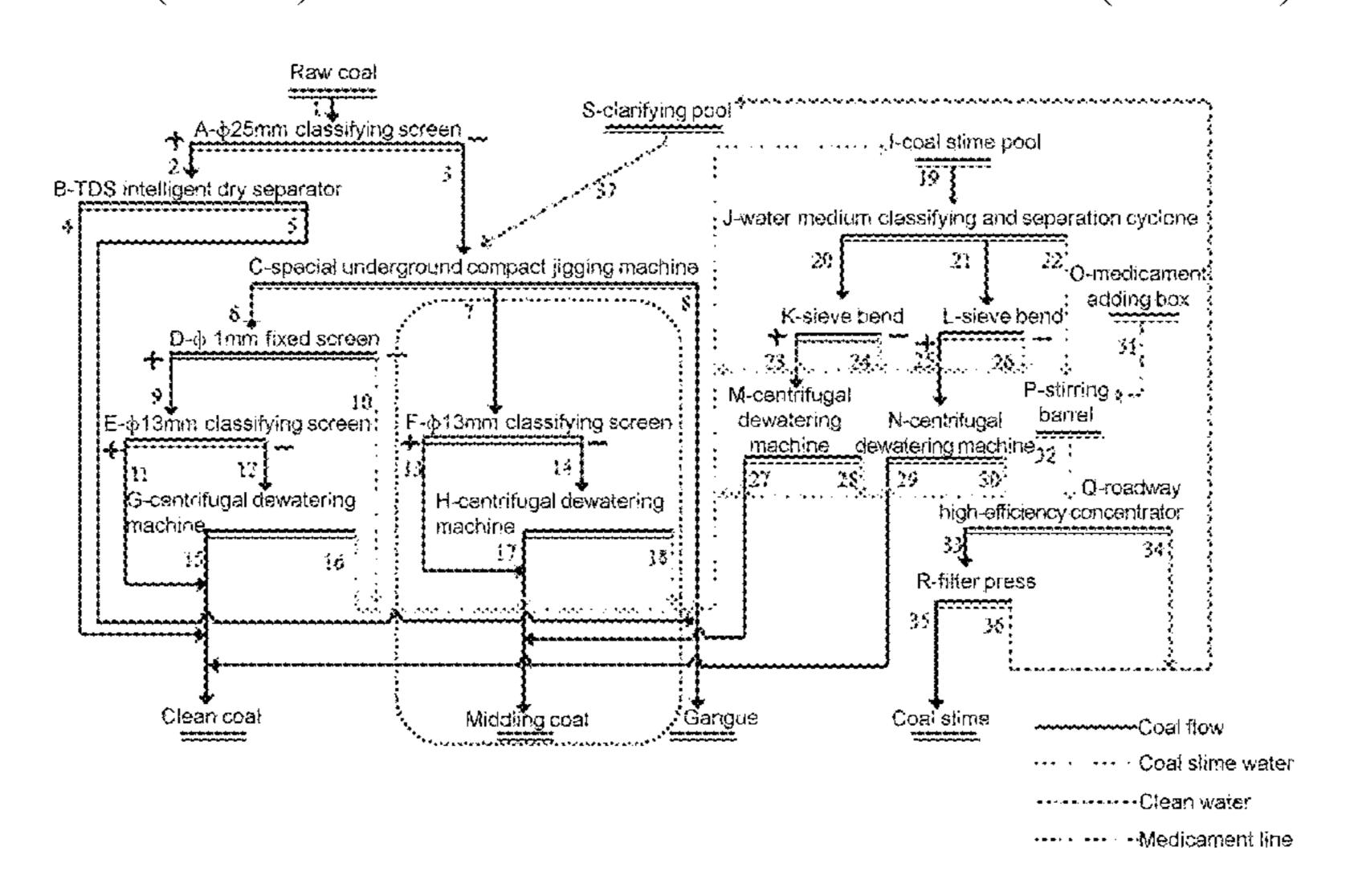
machine overflow clean coal to obtain a clean coal product, and screening and dewatering the jigging middling coal to obtain a middling coal product, sorting slime water to be sorted and generated during sorting to obtain coarse clean coal slime and coarse middling coal slime, and performing circulating water treatment on a final liquid.
