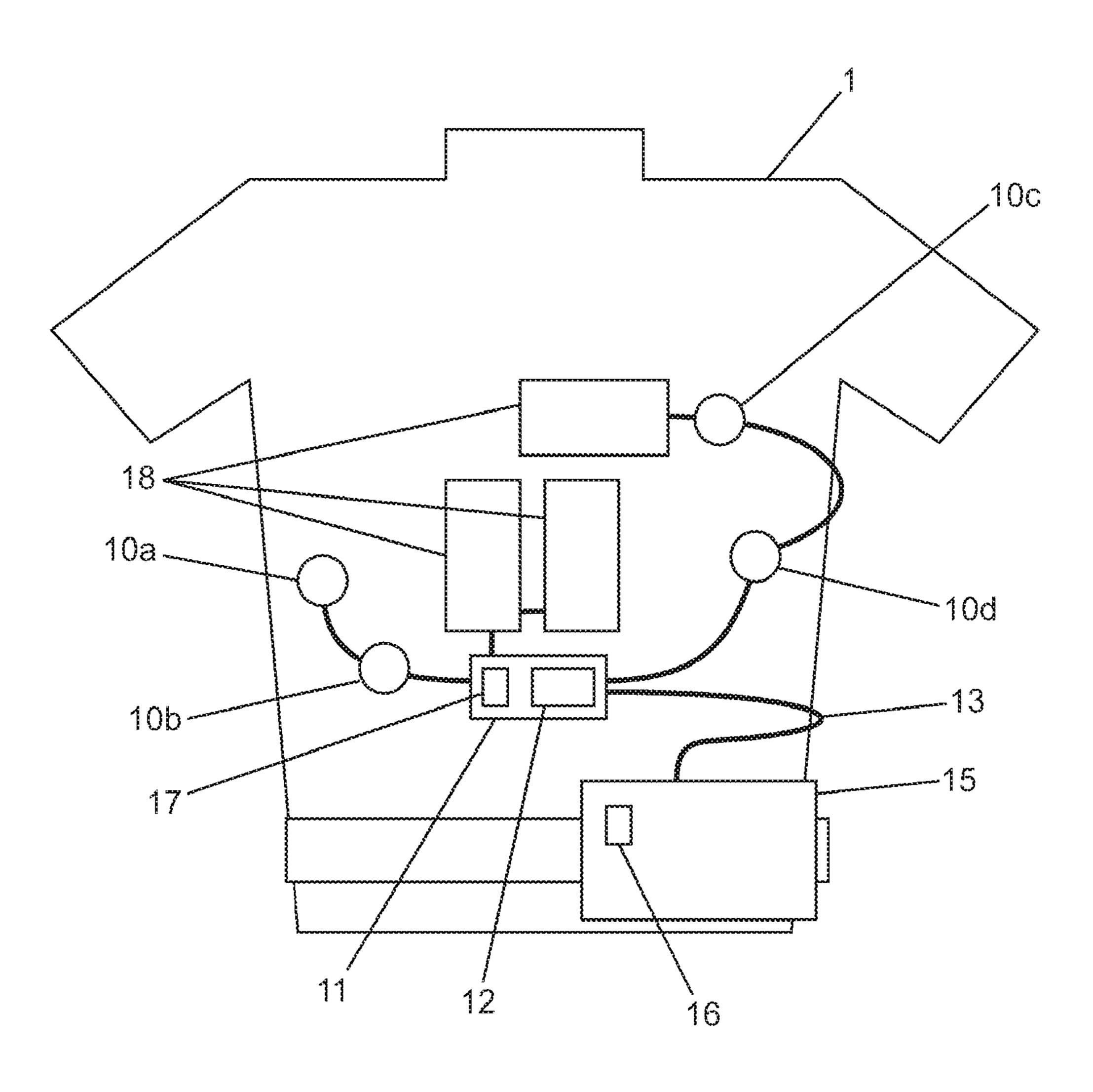
Figure 2: System diagram with accelerometers
