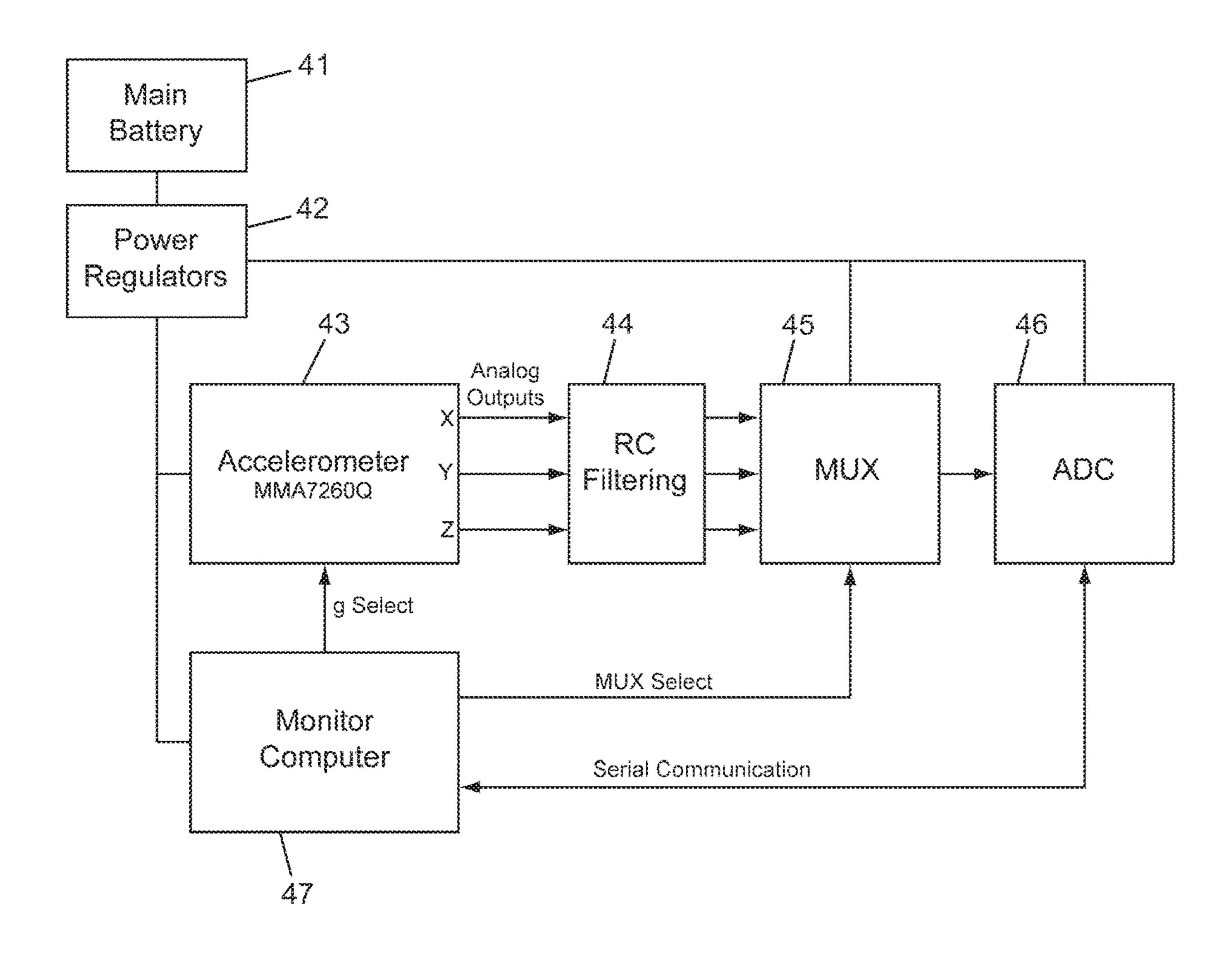
Figure 4: Belt Node Accelerometer
