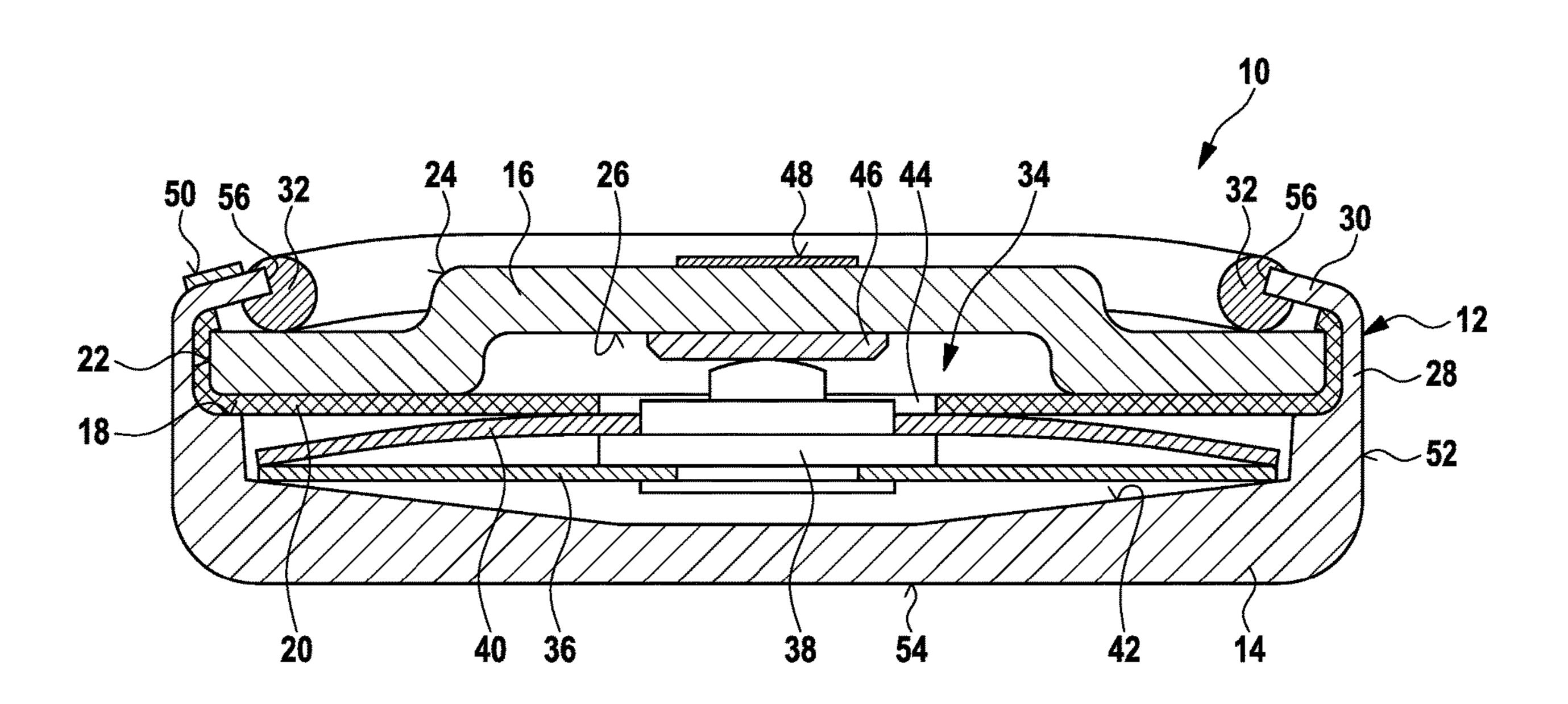
mechanism establishes an electrically conductive connection between the two contact surfaces, and an open state, in which the switching mechanism interrupts the electrically conductive connection between the two contact surfaces. A sealing ring is arranged on the upper side of the cover part, which sealing ring is in sealing contact with the bent upper section of the wall.
