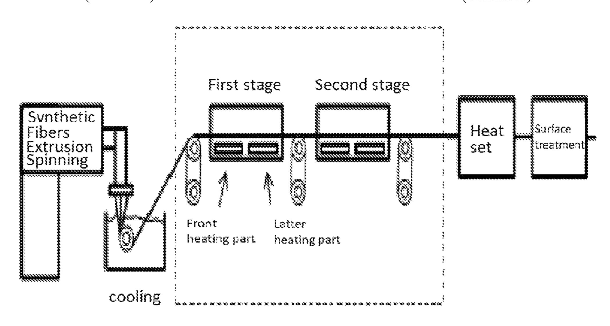
applicable to manufacturing of various types of fibers, enhancing application performance of the fibers.
