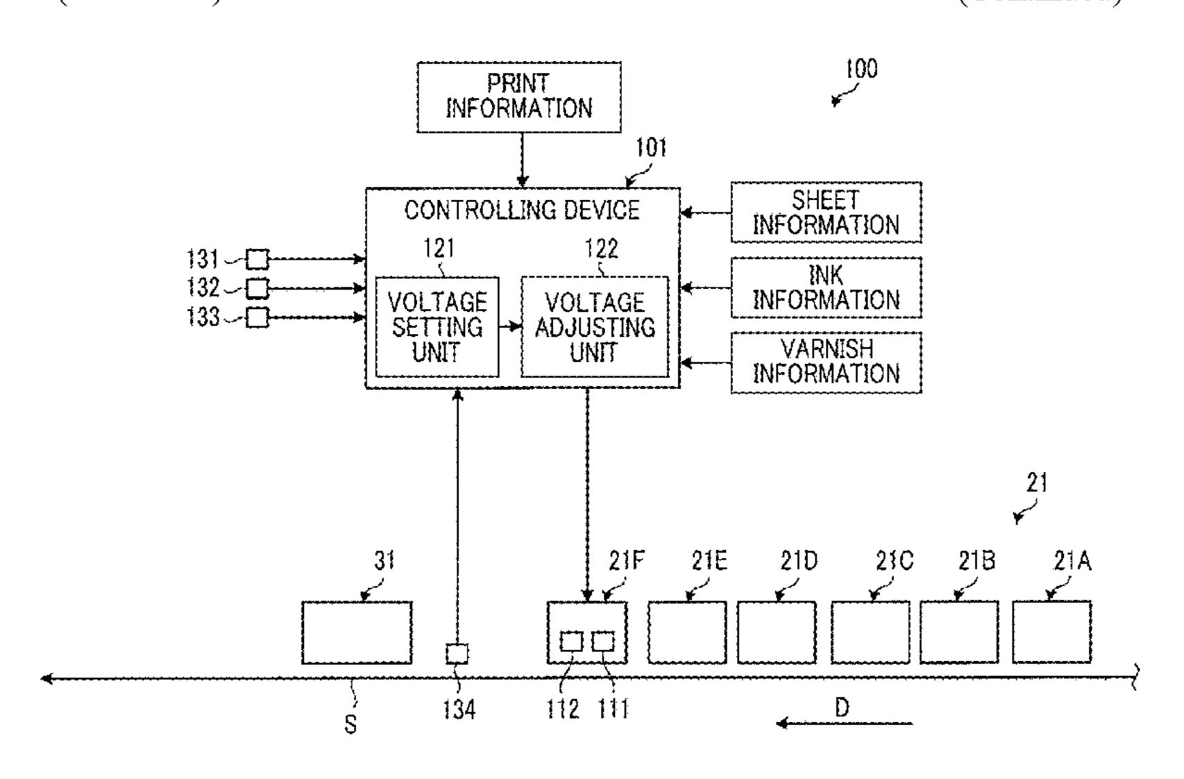
voltage according to the thickness of a water-based paint on the cardboard sheet (S), where the reference voltage is a voltage that is less than the rated voltage of the heating lamp (111) by a preset prescribed value; and a controlling device (101) that changes the voltage of the heating lamp (111) to the working voltage set by the voltage setting unit (121) using the voltage adjusting unit (122).
