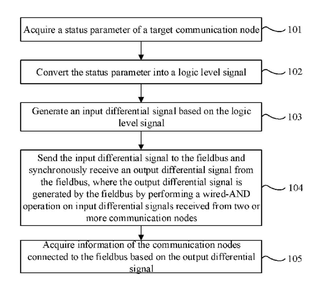
from the two or more communication nodes; and acquiring information of the communication nodes connected to the fieldbus based on the output differential signal.
