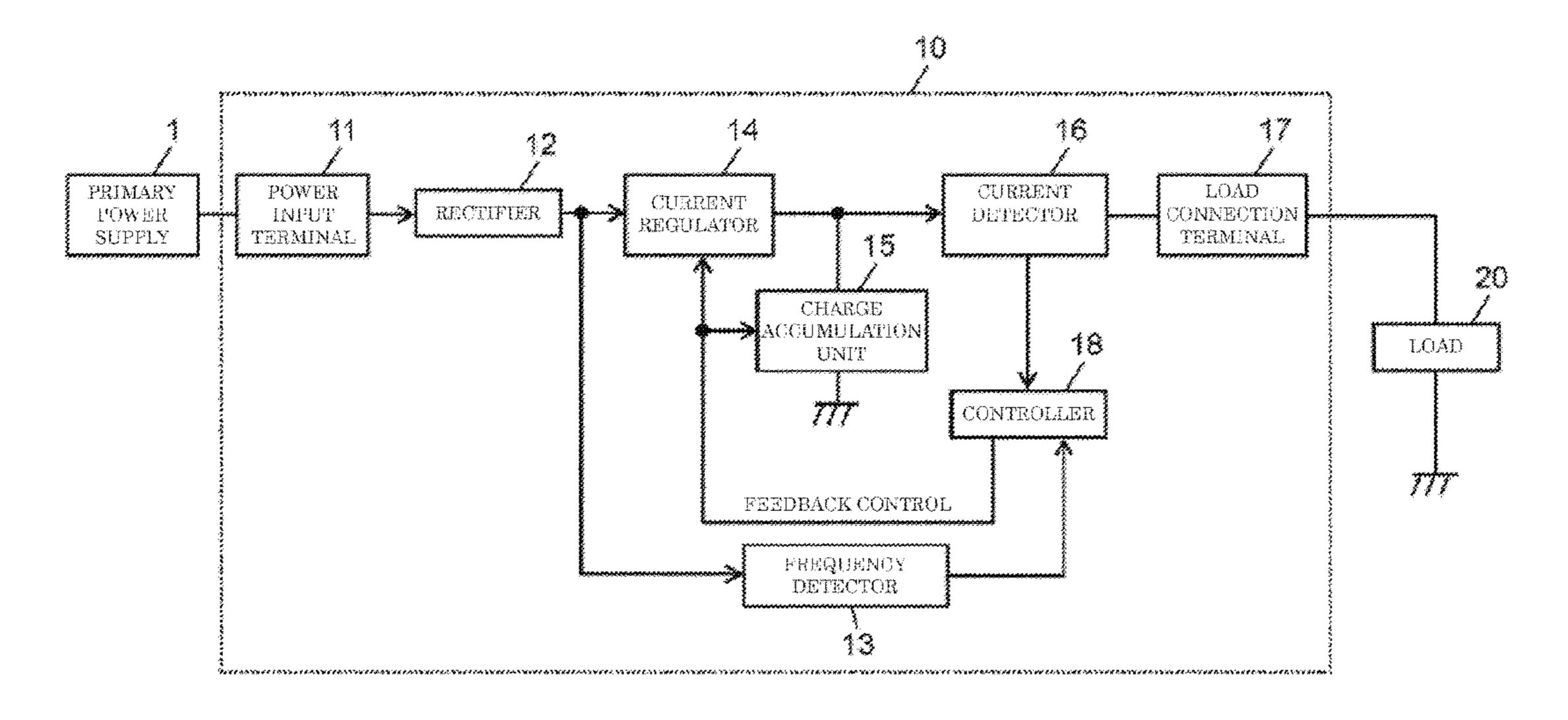
operated by current output from current detector (16), and controller (18) that controls a regulated value of current limiter (14) and capacitance of charge accumulation unit (15) in accordance with fluctuation of the frequency measured by frequency detector (13) in such a manner that the current output from charge accumulation unit (15) becomes larger than current consumed by load (20) at a predetermined time.
