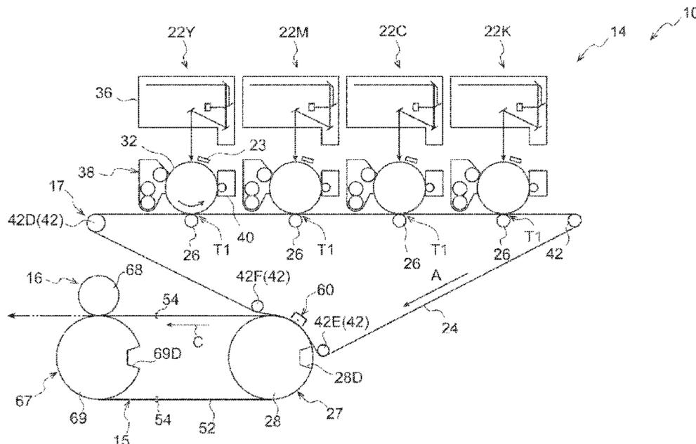
movement of the second nipping part from the first position to the second position is started before a holding position of the recording medium by the holder enters the nip region to when the second nipping part is relatively moved to the first position after the holding position enters the nip region precedes a middle point of a period during which the holding position passes through the nip region.
