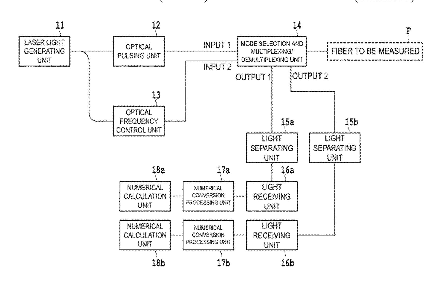
output from the target optical fiber to be measured through the near end to separate light of the first frequency, and a propagation mode loss measuring unit that measures an intensity of the separated light to measure a loss of each propagation mode at each position of the target optical fiber to be measured.
