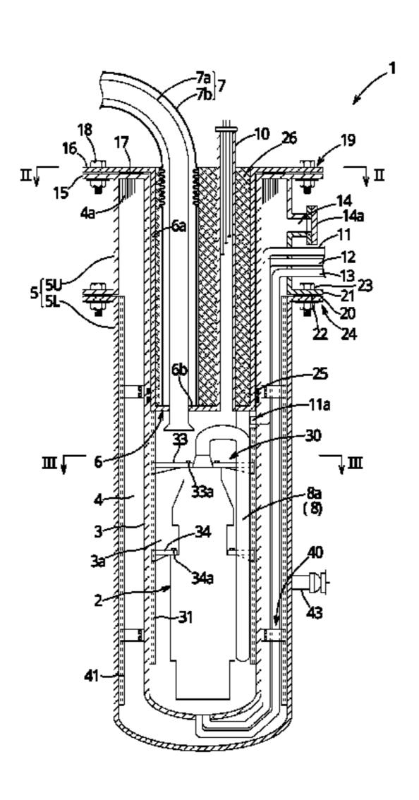
tank. The pump is fixed to the lid structure, and a suction pipe and a discharge pipe are insertedly fixed to the lid structure. A vacuum insulating layer is provided between the inner tank and the outer tank. With this heat insulating vessel for the low temperature liquefied gas pump, adiabaticity of the lid structure and maintainability of the pump are increased.
