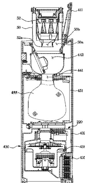
suction the foreign substances and air in the dust collecting chamber docked to the docking station.
