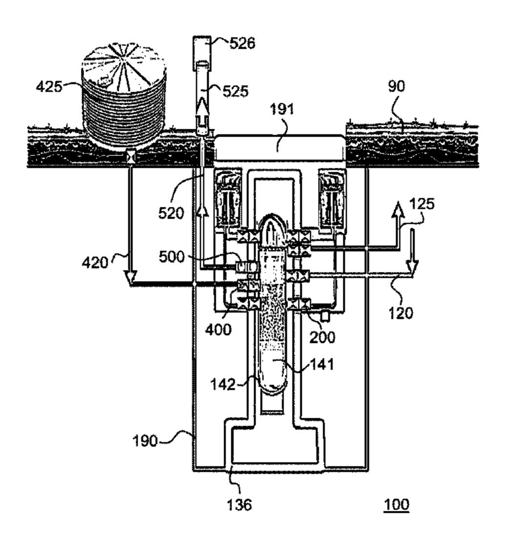
system and injection system together feed-and-bleed coolant through the reactor.
