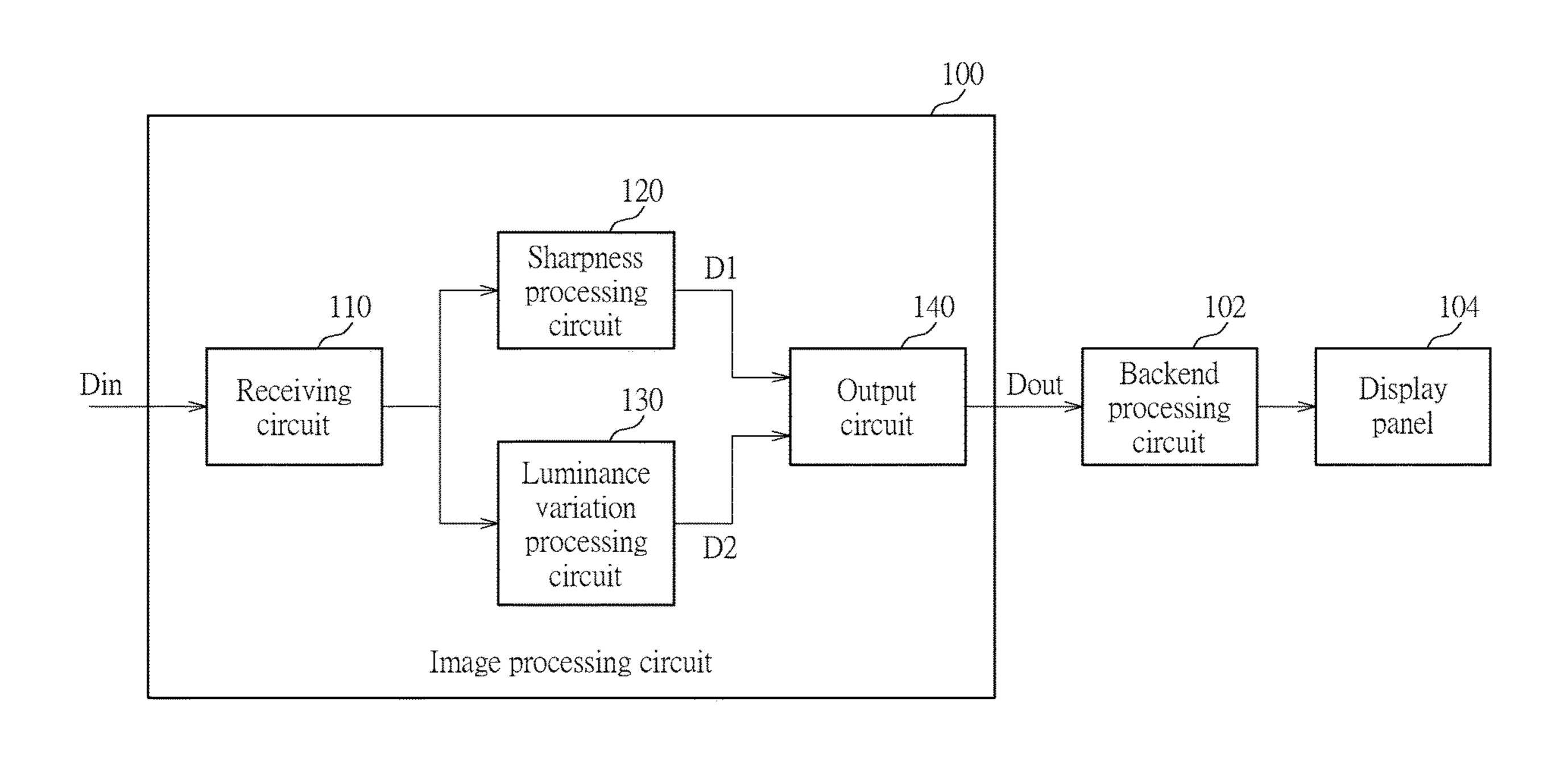
frequency components of the pixel and neighboring pixel(s) to generate auxiliary image data; and the output circuit is configured to generate output image according to the processed image data and the auxiliary image data.
