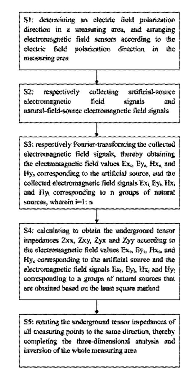
S1: determining an electric field polarization direction in a measuring area, and arranging electromagnetic field sensors according to the electric field polarization direction in the measuring area
