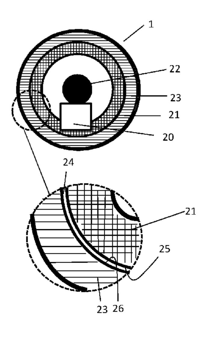
(52, 21) comprises a low friction material having an acoustic impedance in the same order as that of the orbital outer ring **(23)**.
