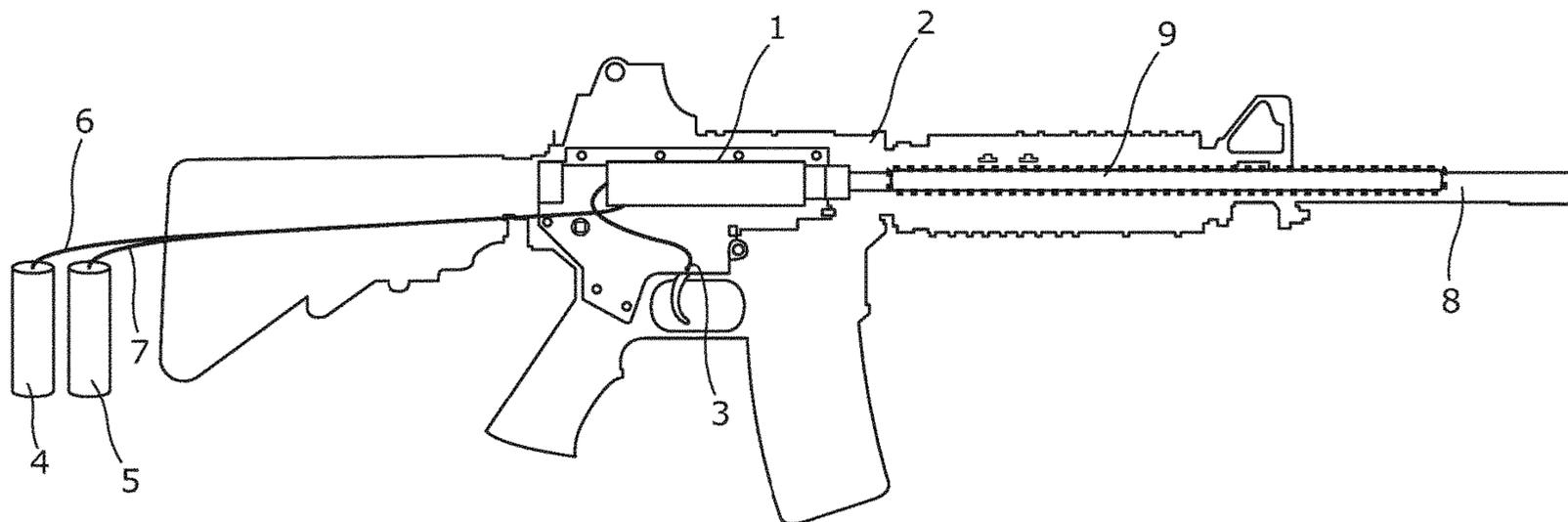
wherein the trigger unit (3) is adapted to activate firing of the firearm by igniting gas in the combustion chamber.
