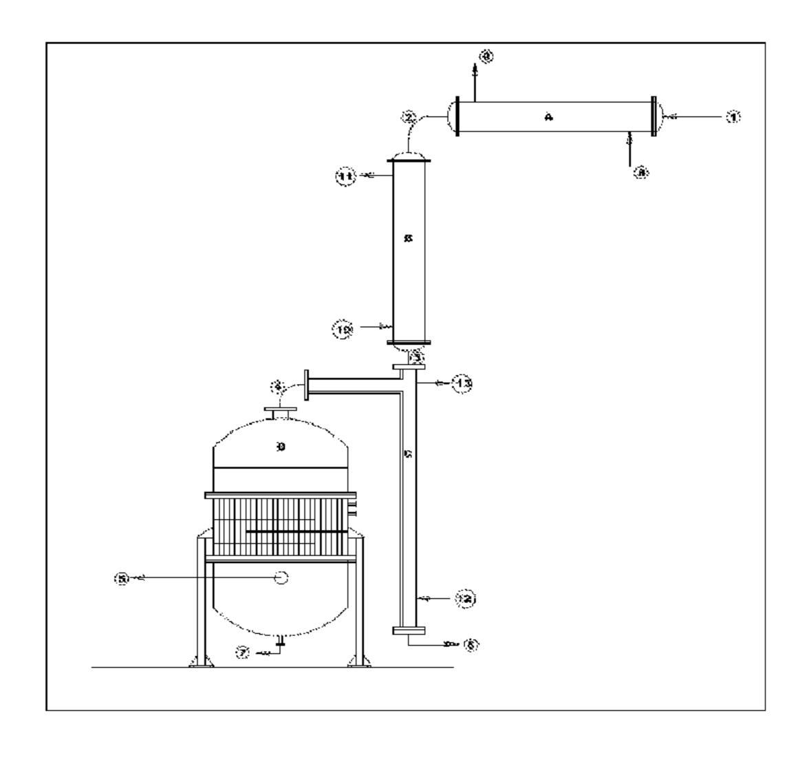
the use of thin film evaporator. The complete transformation of the entire solution of said reactants in to super-heated multicomponent vapor is achieved by heating the entire solution firstly by a pre-heater followed by further heating by a super-heater, further comprising removal of the condensed high boilers and tar to drain, and subjecting the superheated vapor to vapor phase reaction mediated by catalyst to get monoalkyl ether of a dihydric phenolic compound.
