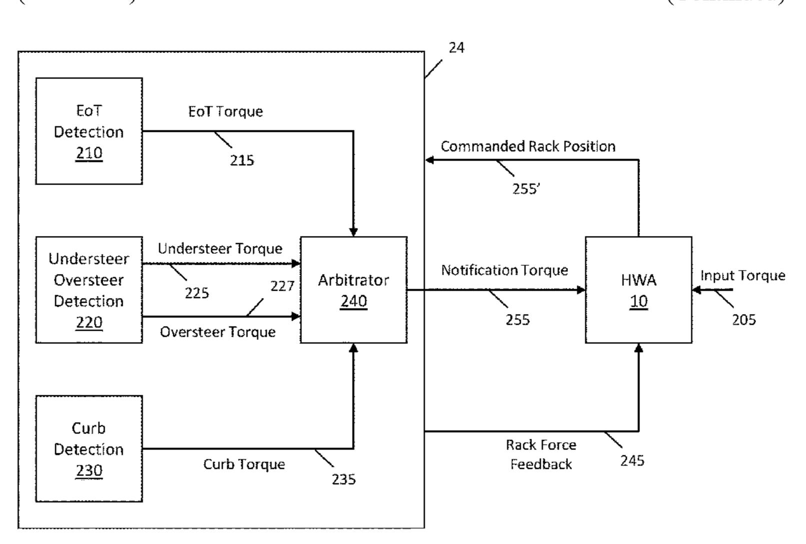
ule that determines a notification torque command by arbitrating between the plurality of torque commands, which comprises the curb torque command and the end-of-travel torque command. The steer-by-wire steering system further includes a second controller that generates a notification torque using the notification torque command.
