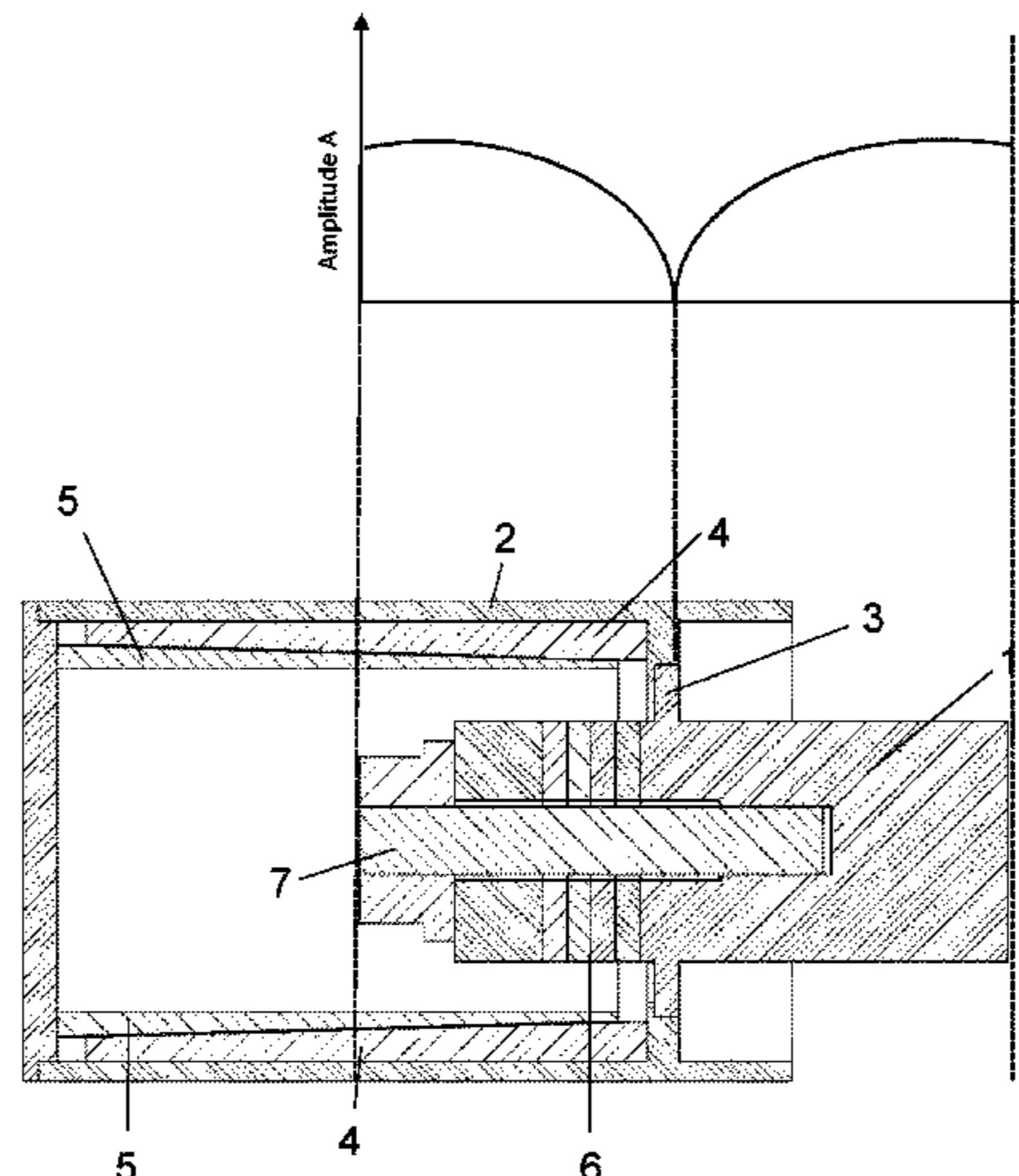
proposed according to the invention that there is provided a damp vibration absorber unit (2) connected to the ultrasonic vibration unit by way of a coupling element (3), wherein the coupling element (3) is connected to the ultrasonic vibration unit at a vibration node, wherein the vibration absorber unit (2) is connected to a damping element (4) which is so adapted that it damps a vibration of the vibration absorber unit (2).
