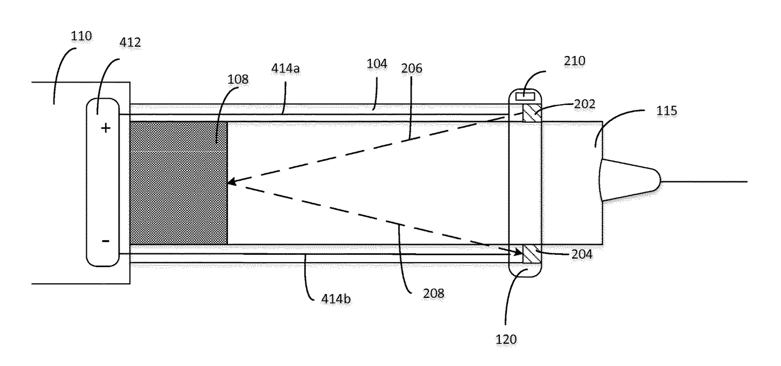
receive reflections of the signal from the stopper, and a controller configured to wirelessly transmit data related to a position of the stopper in the cartridge.
