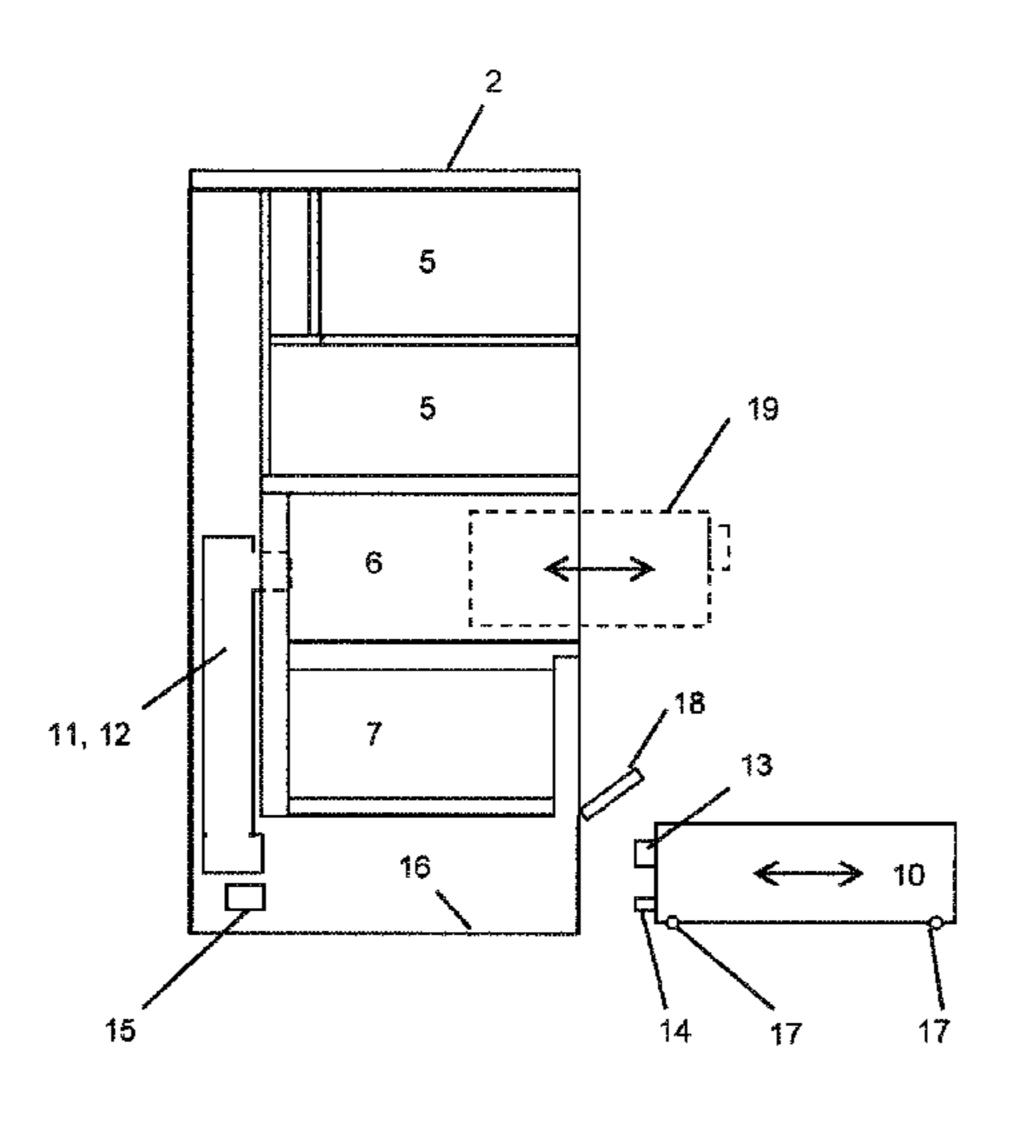
between the at least one environmentally controlled compartment and the environmental control unit, and the environmental control unit having an electric power connector engagable with an electric power outlet in the locker housing in communication with a source of electric power.
