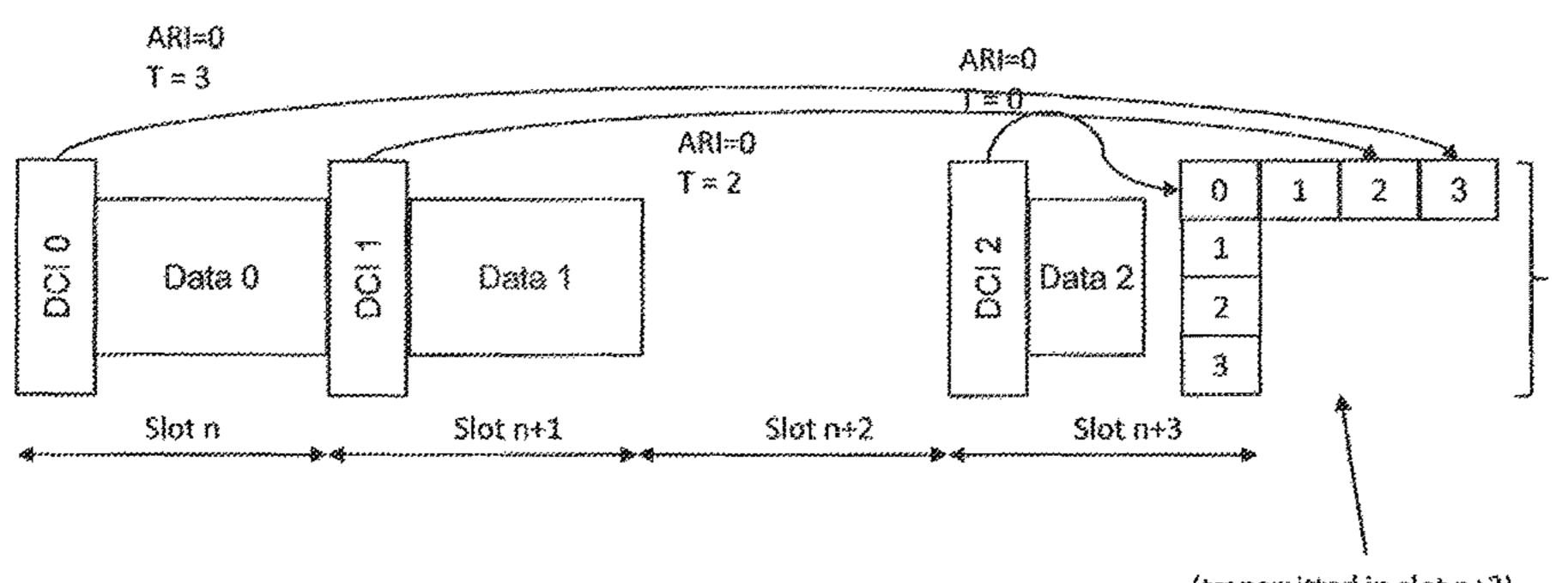
Configured PUCCH resources can be of different payload size, i.e. ARI can select among different PUCCH sizes Timing indicator used to indicate subresources in PUCCH format selected by ARI
