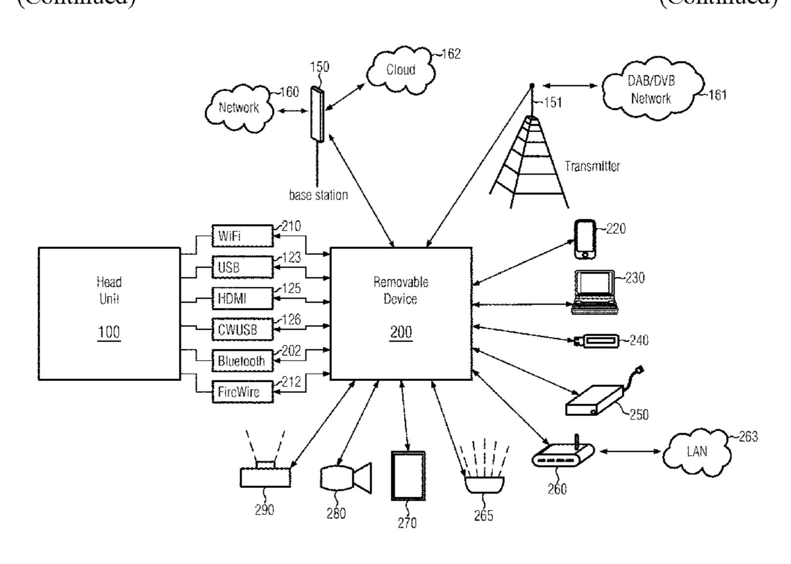
first protocol for the communication with the head unit via the first communication module; and a control unit comprising at least one processing unit adapted to execute the API; wherein the control unit is configured to provide at least one service to the head unit via the first communication module.
