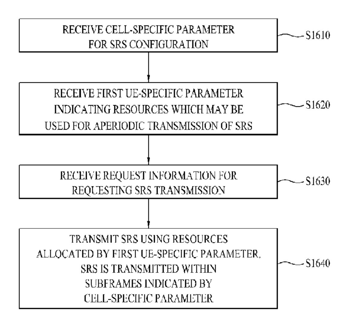
transmission is performed, periodically transmitting the SRS in the configured subframe.
