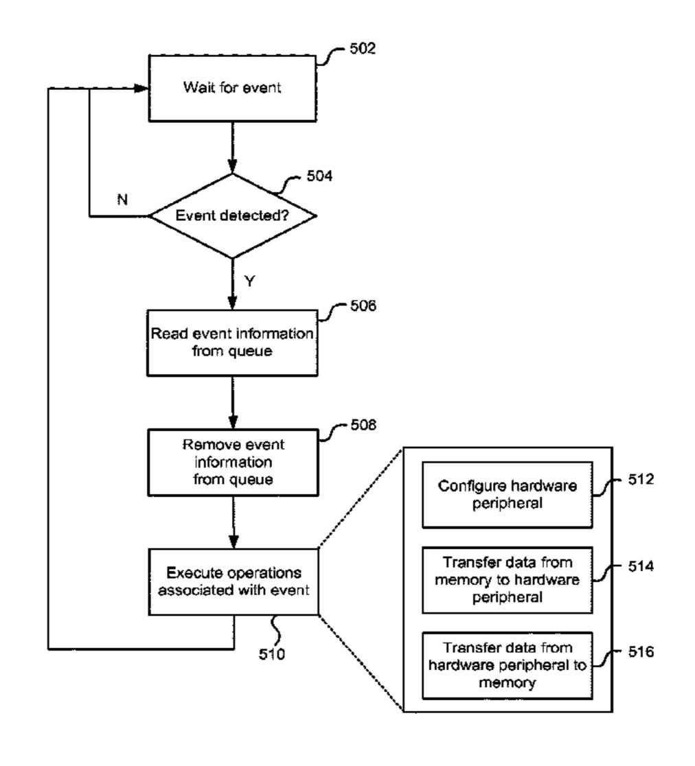
configured to detect an occurrence of an event and, responsive to this, control the memory access controller to enable a selected fixed function accelerator to read data from or write data to the memory device via its memory access channel.
