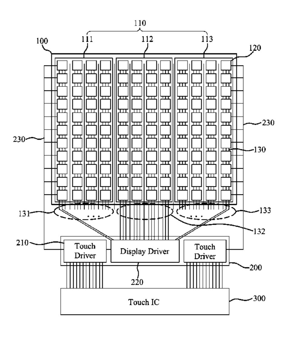
group; and a touch IC configured to generate the touch scan signal and apply the touch scan signal to the display driver IC.
