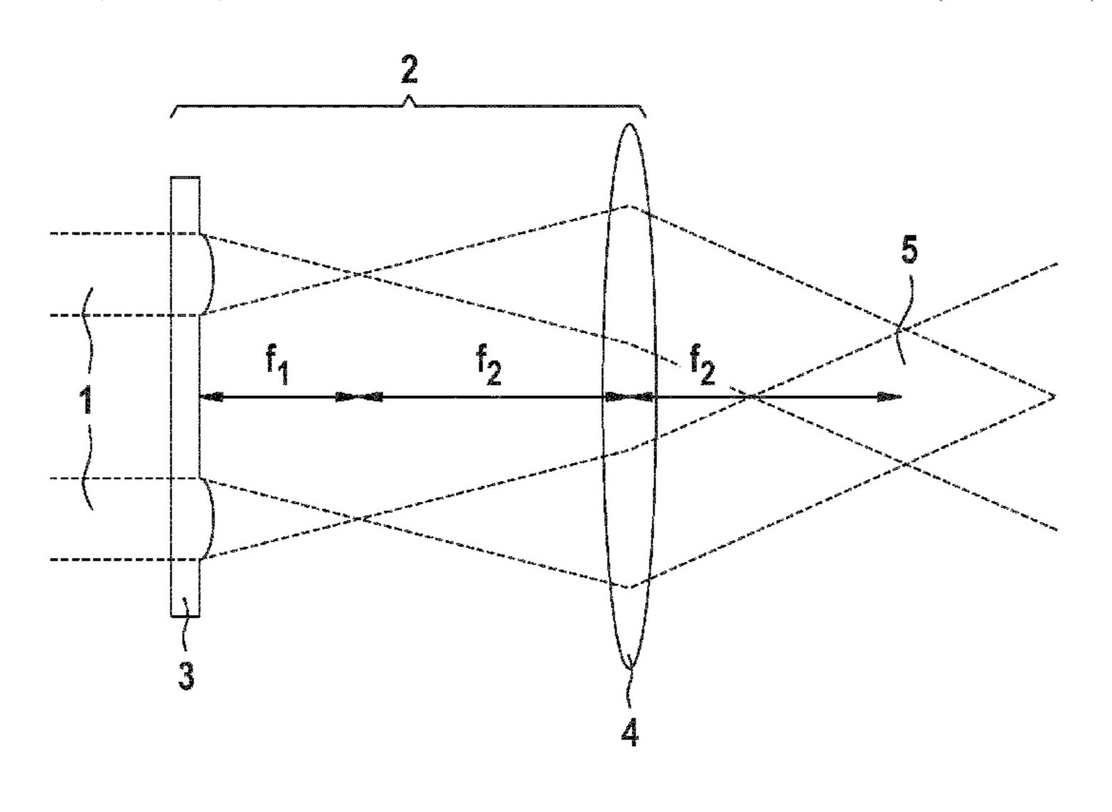
one annular lens (3, 3') and a Fourier optical unit, e.g. in the form of a Fourier lens (4).
