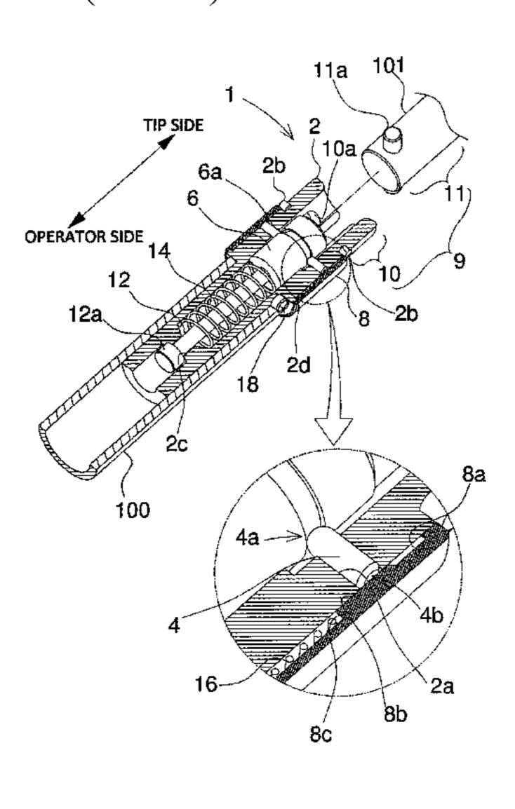
diameter side, wherein an opposing recess which can oppose to the recessed grove is formed on the outer slider.
