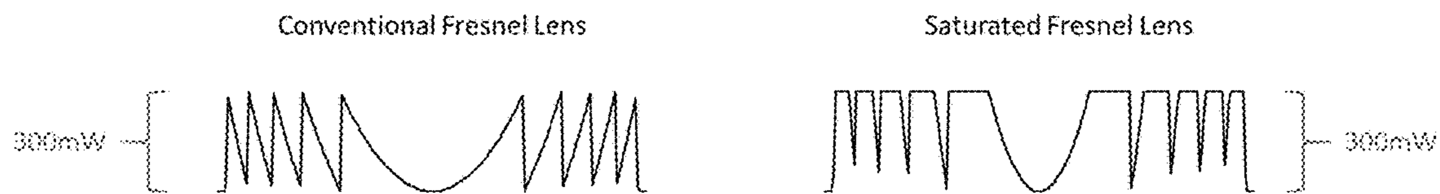
Figure 4. Conventional (left) and saturated (right) Fresnel lenses shown in cross-section with equal height of 300mW.
