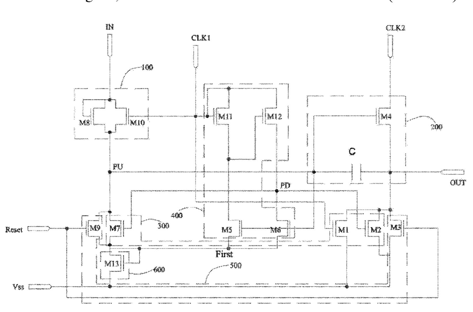
under control of a signal from the second signal terminal. The pull-down sub-circuit conducts the pull-up node with the first node and the turn-down signal terminal with the output terminal under control of a potential of the pull-down node. The voltage regulating sub-circuit conducts the first node with the turn-down signal terminal under control of a potential of the first node.
