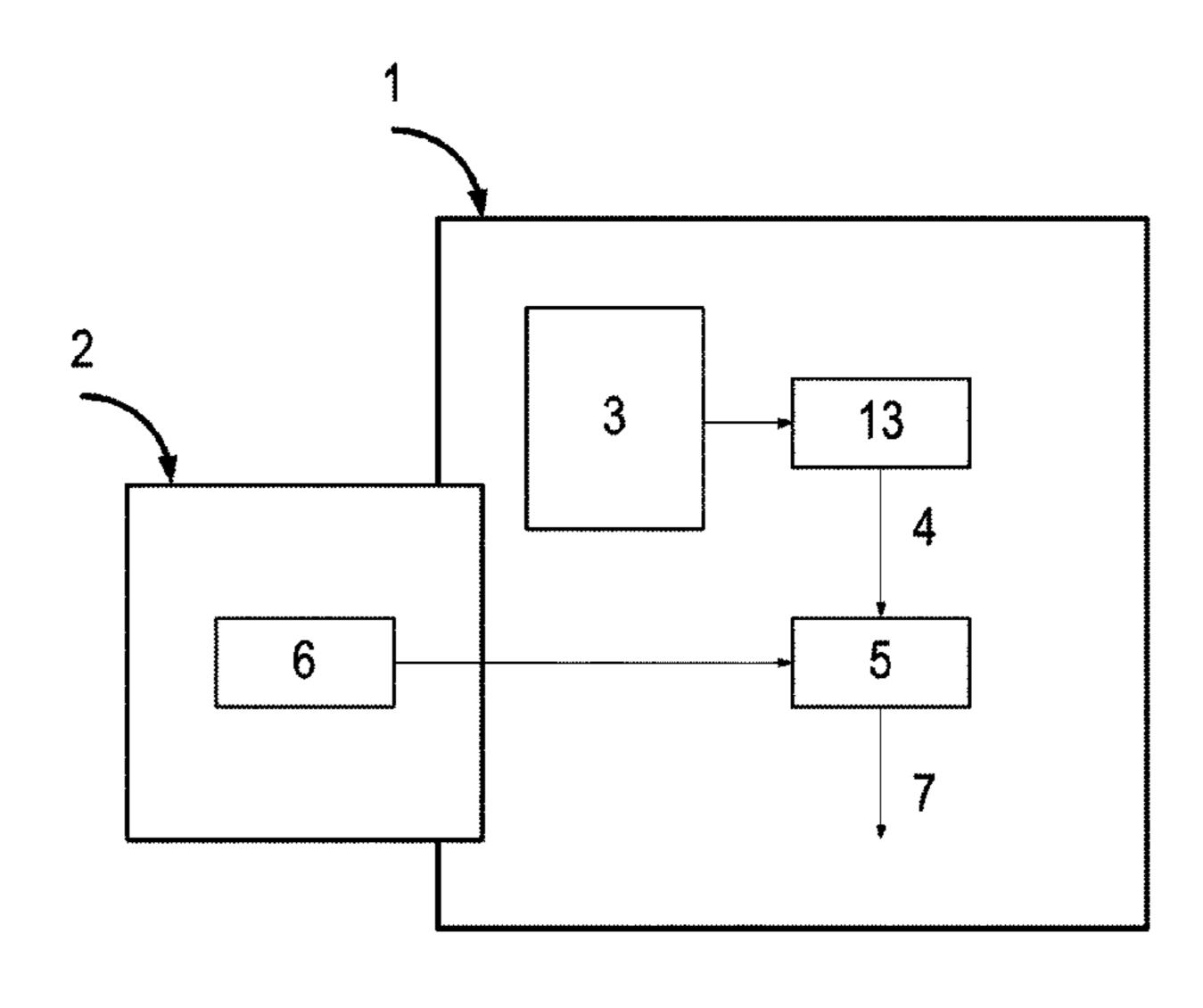
interface being spatially restricted, and the key memory being location-bound. The security device includes at least one calculation unit, which dynamically ascertains in particular the check-sum information from the parameter data record.
