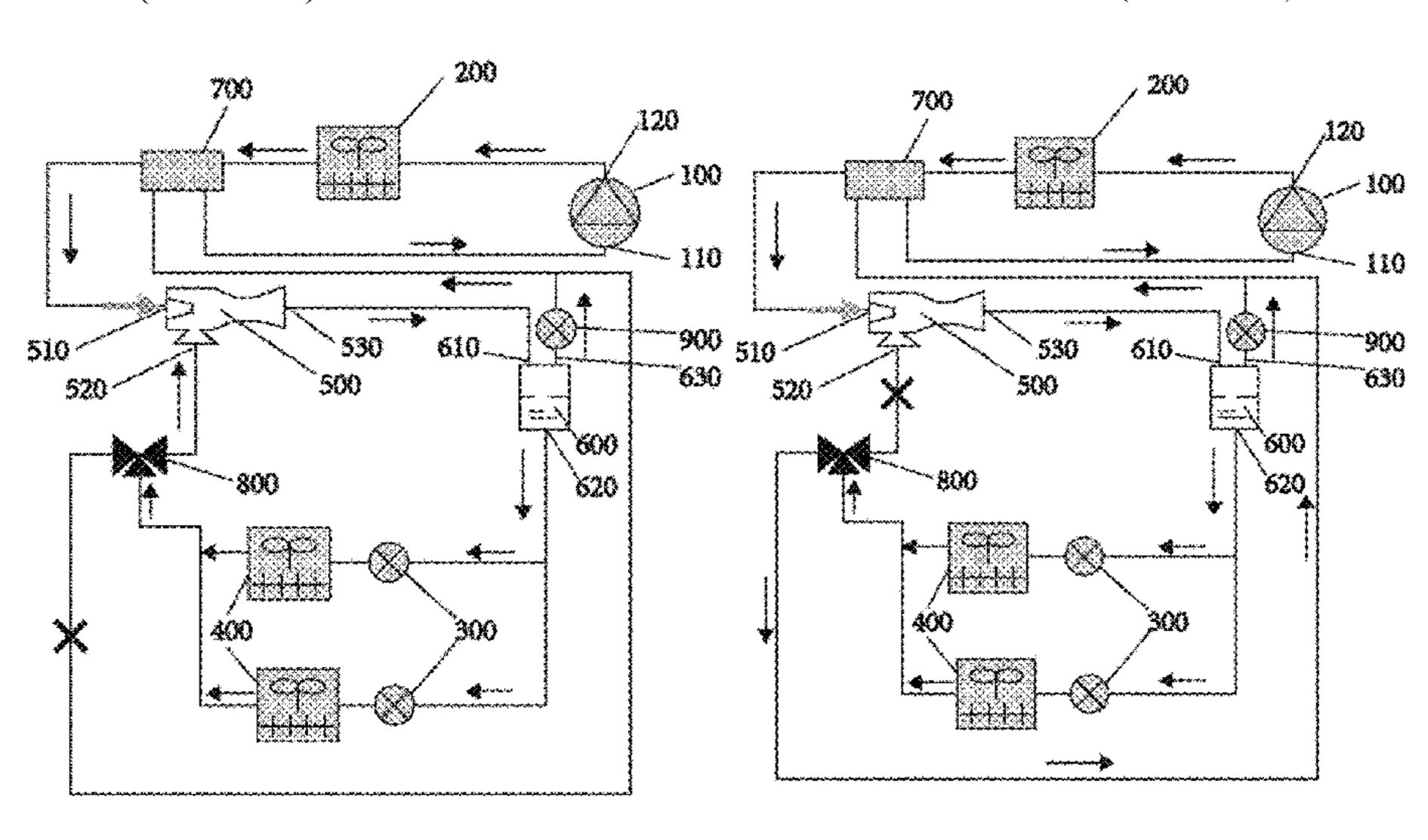
second flow path connecting the heat-absorption heat exchanger and the gas inlet of the compressor are controllable.
