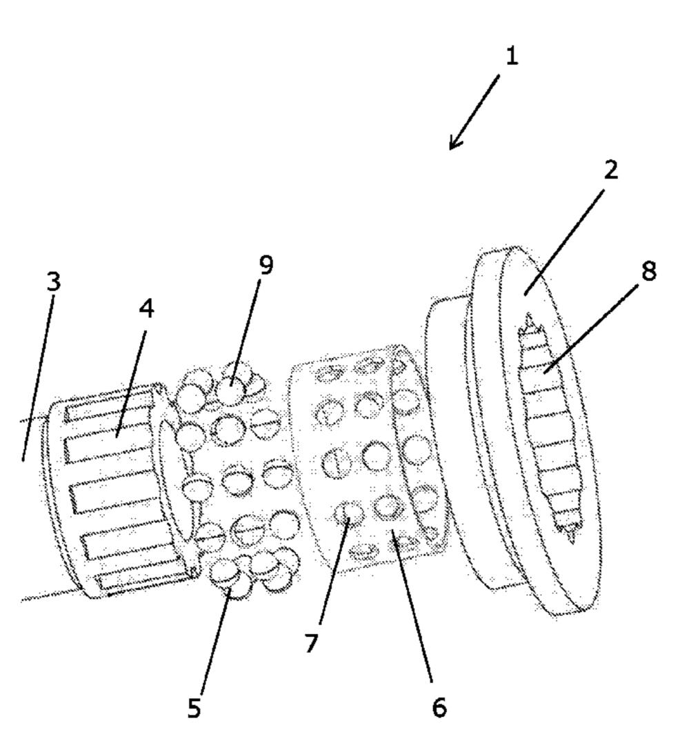
direction of shaft (3). The through-going openings (7) in the insulating cage (6) are arranged aligned with the plurality of first grooves (4) and the plurality of second grooves (8). The insulating members (5) are arranged in the through-going openings (7) of the insulating cage (6) and in the first and second grooves, so as to be adapted to transfer torque from the shaft to the rotational member (2) via the insulating members (5).
