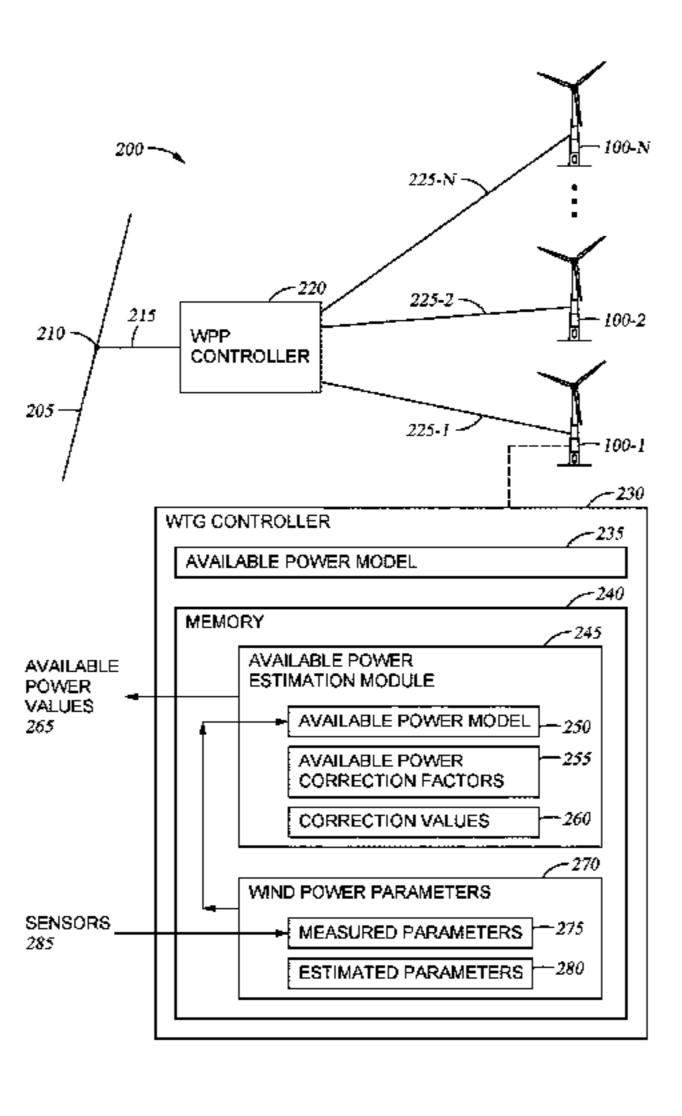
applied to a predefined model for estimating an available power of the wind turbine, an estimated available power value; adjusting the estimated available power value using the one or more available power correction factors to produce the available power value; and controlling, using the available power value, the wind turbine to produce a second power production level.
