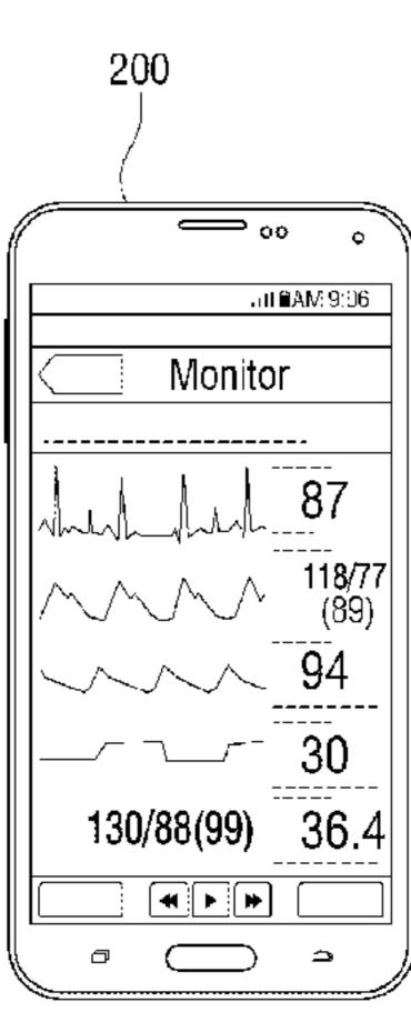
The electronic device, according to one embodiment of the present disclosure, comprises: a sensor for measuring a biological signal of a user; and a processor for determining the periodicity of the measured biological signal, and selectively compressing the measured biological signal according to the determined periodicity.
