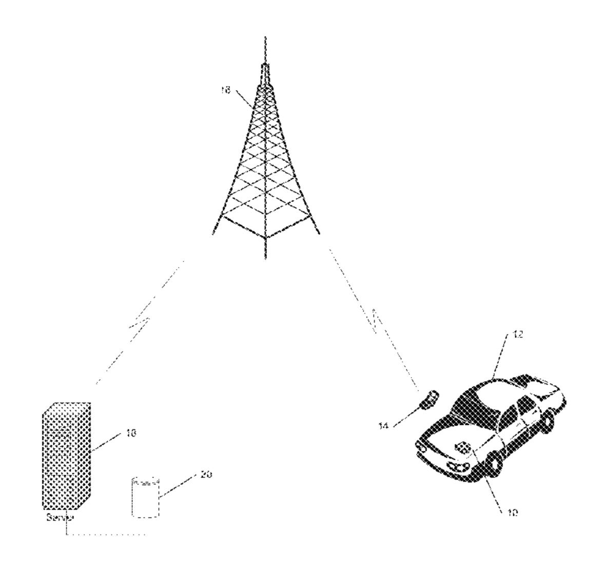
device obtains GPS data, combines this with the acceleration date and transmits this to a server for analysis.
