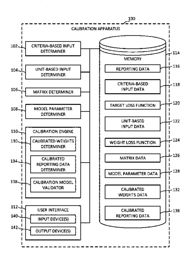
calibration model validator to incorporate a stability parameter into the calibration model in response to determining that the calibrated weights do not provide a unique solution for the executed calibration model. The stability parameter is to reduce an influence of the budget parameter on the calibration model to enable the generation of a unique solution.
