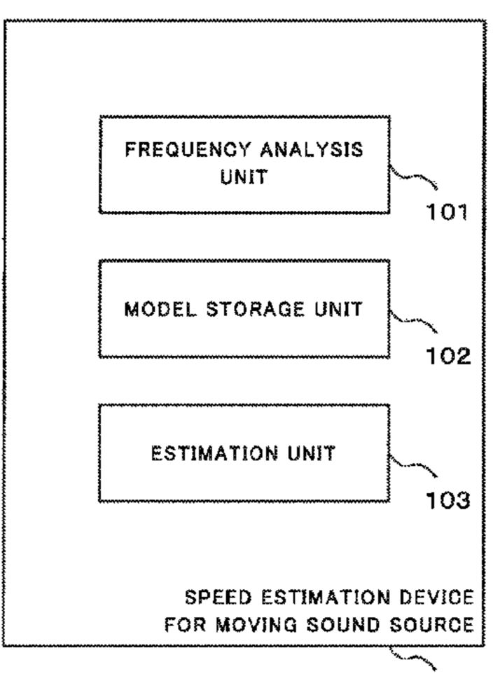
estimation unit (103) estimates the movement speed of the sound source on the basis of the spectrogram generated by the frequency analysis unit (101) and the plurality of spectrograms indicated by the spectrogram template information stored in the model storage unit (102).
