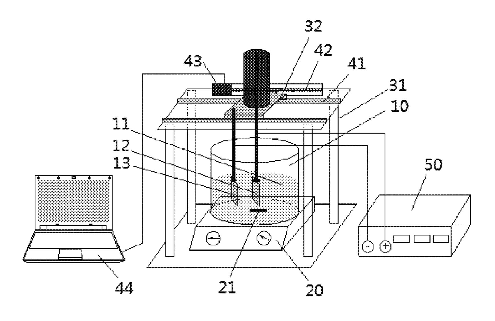
nano-metal oxide film. The film preparation method according to the disclosure offers advantages such as mild condition, simple instrumentation, easy operation, and low cost; the prepared film has a good load effect such that the metal oxide can hardly be shed off.
